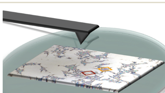
Fig. 1 A schematic illustration of the AFM experimental setup displaying the two different regions being investigated. Images were scanned from both the periphery (red), i.e. the chains on the particle surface, and the denser region (orange).
