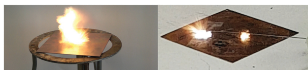
Fig. 20 Detonation of compound 5a during hot plate test (right side) and detonation of complex 10 (left side).
