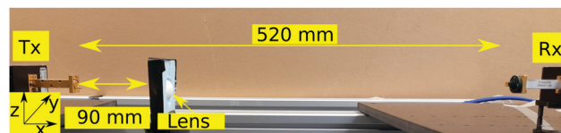
Fig. 3 Measurement setup to measure electric field deflected by the lens. The lens is inside a foam holder which is supported by a rod which can be moved in x -, y -, z -directions by stepper motors between the transmitter (Tx) and receiver (Rx). As the lens is the only moving part, the recorded intensity of the S_{21} does not have false readings ( i.e. , intensity changes) caused by cable movements.
