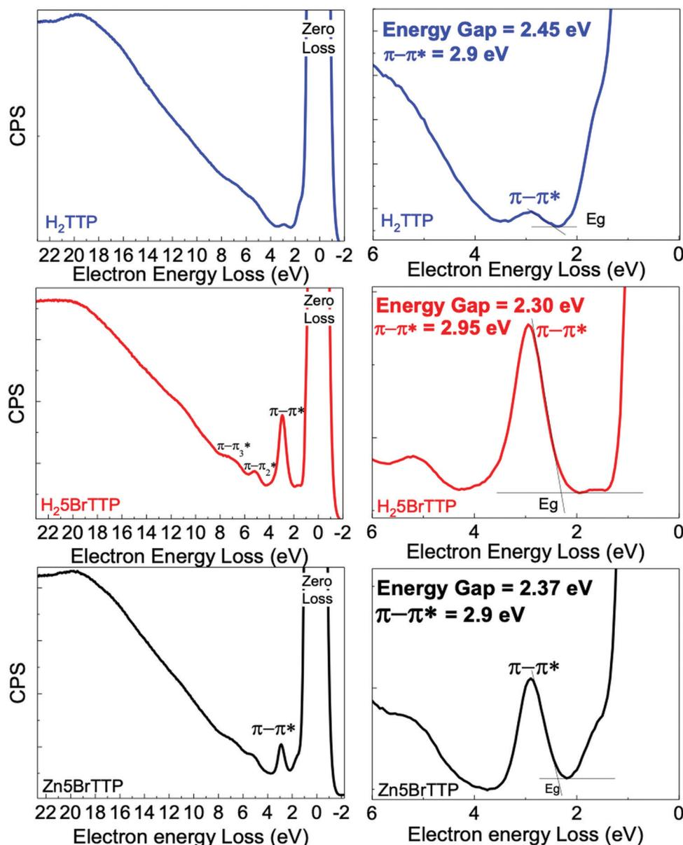
Fig. 1 REELS spectra of H<sub>2</sub>TTP, H<sub>2</sub>5BrTTP and Zn5BrTTP thin films (deposited over ITO/glass substrate). The left side is an overall view. The right side shows the determination of the electronic energy gap ( $E_g$ ).
