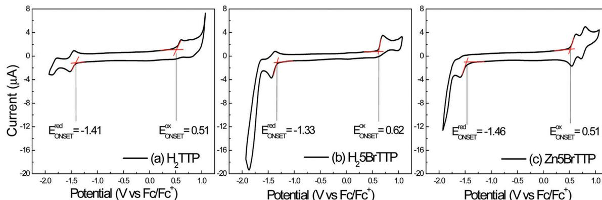
Fig. 2 Voltammograms for the three porphyrin derivatives: (a) **H<sub>2</sub>TTP**, (b) **H<sub>2</sub>5BrTTP** and (c) **Zn5BrTTP**, from which the electrochemical energy gap can be obtained by considering the difference between oxidation and reduction potentials. The red lines highlight the onset considered to extract the redox potentials values.
