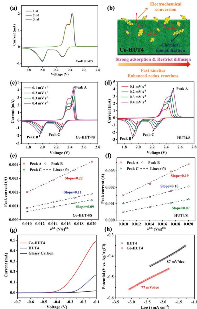
Fig. 6 (a) CV curves of Co-HUT4 in the initial three cycles at  $0.1 \text{ mV s}^{-1}$ ; (b) schematic illustration of LiPS conversion on the surface of the Co-HUT4 porous framework; CV curves at different scan rates of (c) Co-HUT4/S and (d) HUT4/S electrode; (e and f) the corresponding linear fitting in the light of Randles-Sevcik equation; (g) LSV curves of  $\text{Li}_2\text{S}_2$  oxidation; (h) the corresponding Tafel plots of HUT4 and Co-HUT4.
