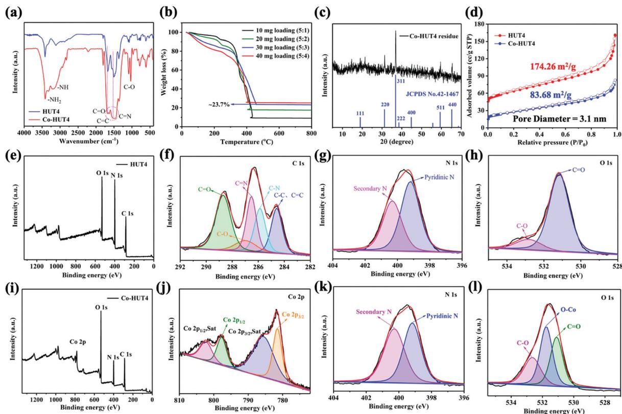
Fig. 4 (a) FT-IR spectra of HUT4 and Co-HUT4; (b) TGA curves of Co-HUT4 in O<sub>2</sub>; (c) PXRD pattern of the residue left; (d) comparative N<sub>2</sub> adsorption isotherms of HUT4 and Co-HUT4; (e) the XPS survey spectrum; (f) C 1s; (g) N 1s and (h) O 1s XPS spectra of HUT4; (i) the XPS survey spectrum; (j) Co 2p; (k) N 1s; (l) O 1s XPS spectra of Co-HUT4.
