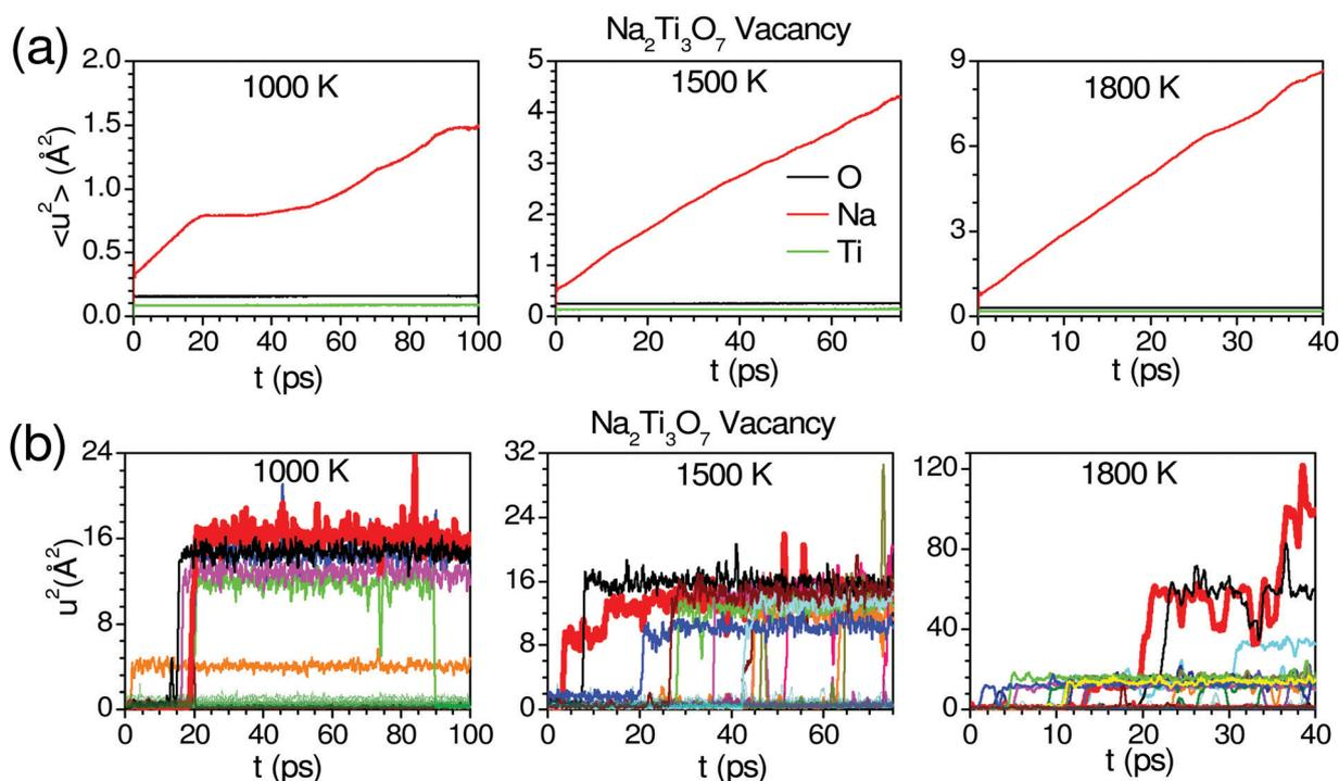
Fig. 3 (a) Time-dependent mean-squared displacements (MSD;  $\langle u^2 \rangle = \langle u_x^2 \rangle + \langle u_y^2 \rangle + \langle u_z^2 \rangle$ ), for various atoms in Na<sub>2</sub>Ti<sub>3</sub>O<sub>7</sub> with one Na vacancy in a (3 × 2 × 2) supercell. (b) The calculated  $u^2$  of individual Na atoms is represented by different colors. The 3-d trajectories of selected Na atoms (marked by a thick red line) are shown in Fig. 4.
