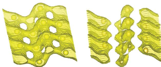
**Fig. 7** The bond valence energy landscape (BVEL) map of  $\text{Na}_2\text{Ti}_3\text{O}_7$  as estimated from the structural data<sup>35</sup> at 300 K. Left and right figures correspond to the iso-energy surface of 0.34 eV and 0.20 eV, respectively. The yellow spheres show the equilibrium positions of Na. The map is shown in the  $a$ - $c$  plane, where the  $a$ -axis is along the one-dimensional channel formed by Na atoms.
