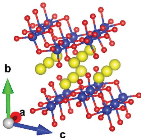
Fig. 1 Crystal structure of  $\text{Na}_2\text{Ti}_3\text{O}_7$ . The color scheme is Ti: blue, Na: yellow and O: red. The lattice parameters of the monoclinic unit cell are:  $a = 3.8008 \text{ \AA}$ ,  $b = 8.5602 \text{ \AA}$ ,  $c = 9.1252 \text{ \AA}$ , and  $\alpha = 101.598^\circ$ .
