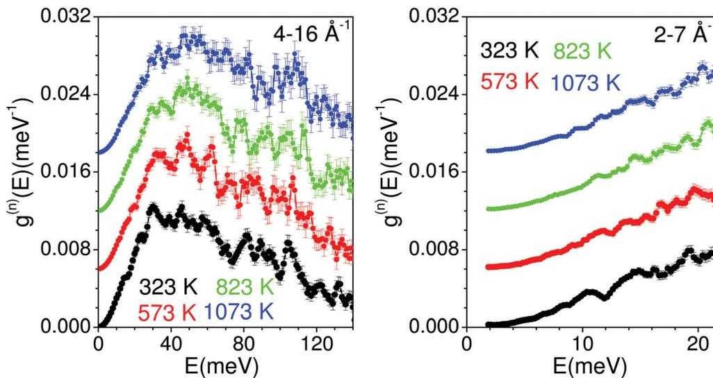
Fig. 8 The experimentally measured neutron-weighted phonon density of states in  $\text{Na}_2\text{Ti}_3\text{O}_7$  at various temperatures. The multi-phonon contribution has been corrected using a standard procedure at ISIS.
