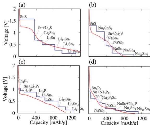
**Fig. 2** The voltage–capacity curves of (a) Li/SnS, (b) Na/SnS, (c) Li/Sn<sub>4</sub>P<sub>3</sub> and (d) Na/Sn<sub>4</sub>P<sub>3</sub> systems as negative electrodes (blue solid lines). The experimental values of the first discharge processes (red solid lines) were taken from ref. 39 (Li/SnS), 27 (Na/SnS), 42 (Li/Sn<sub>4</sub>P<sub>3</sub>), and 43 (Na/Sn<sub>4</sub>P<sub>3</sub>).
