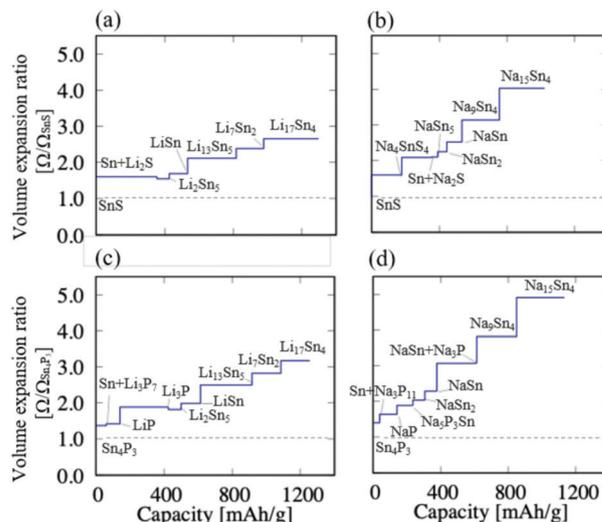
Fig. 3 The volume expansion ratios of (a) Li/SnS, (b) Na/SnS, (c) Li/Sn<sub>4</sub>P<sub>3</sub> and (d) Na/Sn<sub>4</sub>P<sub>3</sub> as negative electrodes.
