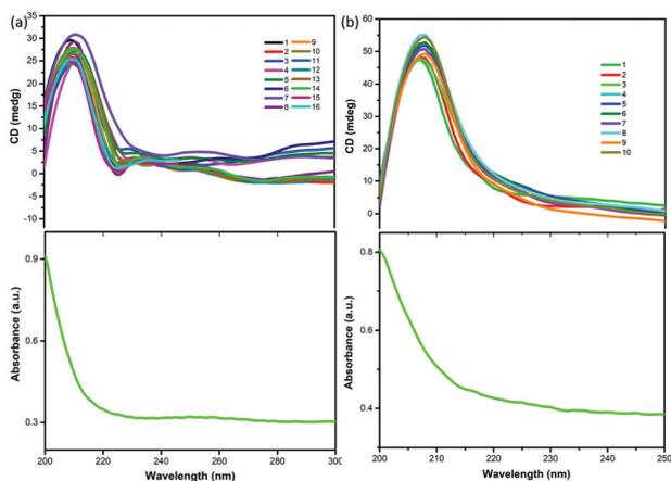
Fig. 7 Solid-state CD spectra of compounds **1** (a) and **2** (b) and the corresponding absorption spectra at room temperature.
