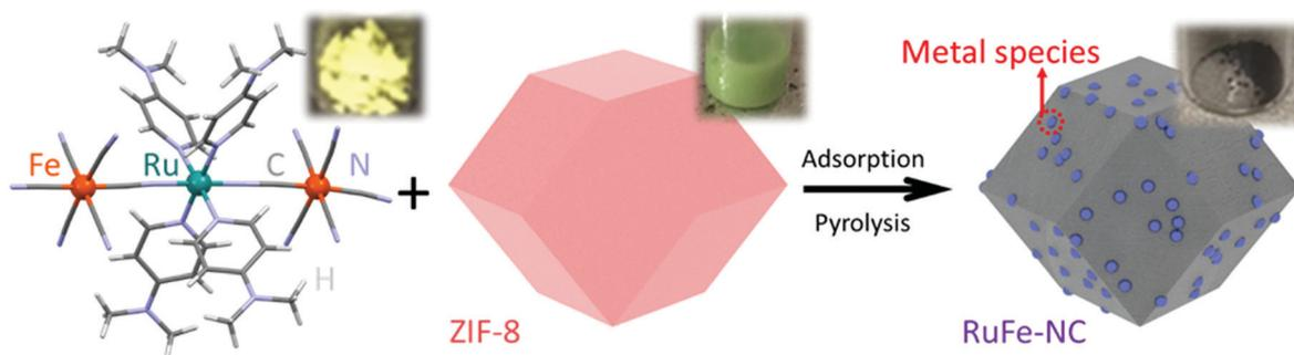
Scheme 1 Molecular structure of the Ru(LFe)<sub>2</sub> complex and the synthetic procedure of the RuFe-NC composite. Insets show the photographs of the products at different reaction stages.
