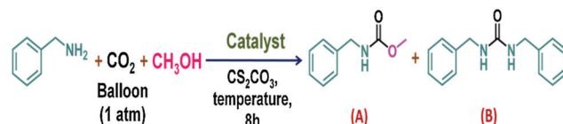
Scheme 28 Methyl benzyl carbamate synthesis via a CO 2 fixation reaction. Reproduced with permission from ref. 54; copyright: 2020, Molecular Catalysis.
