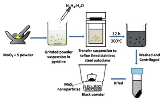
Fig. 7 Preparation of MoS<sub>2</sub> NPs in an autoclave using MoO<sub>3</sub> (ref. 59).
