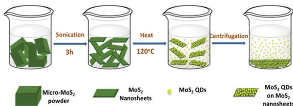
Fig. 16 Illustration of reaction steps for sonochemical synthesis of MoSe<sub>2</sub> QDs and nanosheets. Reprinted with permission from ref. 110 [S. Xu, D. Li and P. Wu, *Adv. Funct. Mater.*, 2015, **25**, 1127–1136]. Copyright WILEY-VCH Verlag GmbH & Co. KGaA, Weinheim.
