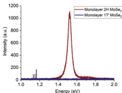
Fig. 13 PL spectra of monolayer 2H and 1T'-MoSe<sub>2</sub>. Reprinted with permission from ref. 93 [E. D. Hanson, L. M. Lilley, J. D. Cain, S. Hao, E. Palacios, K. Aydin, C. Wolverton, T. Meade and V. P. Dravid, *Mater. Chem. Phys.*, 2019, **225**, 219–226]. Copyright 2019, Elsevier.
