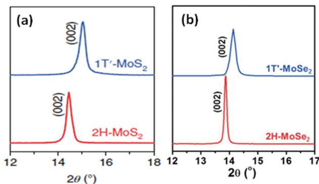
Fig. 22 Variation in XRD peaks depending upon the phase of the (a) MoS<sub>2</sub> and (b) MoSe<sub>2</sub> compounds. Reprinted with permission from ref. 23 [Y. Yu, G. H. Nam, Q. He, X. J. Wu, K. Zhang, Z. Yang, J. Chen, Q. Ma, M. Zhao, Z. Liu, F. R. Ran, X. Wang, H. Li, X. Huang, B. Li, Q. Xiong, Q. Zhang, Z. Liu, L. Gu, Y. Du, W. Huang and H. Zhang, *Nat. Chem.*, 2018, **10**, 638–643]. Copyright 2018, The Author(s).
