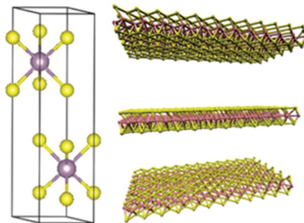
Fig. 2 Crystal structure of 2H-MoSe<sub>2</sub> Reprinted with permission from ref. 27 [S. Tongay, J. Zhou, C. Ataca, K. Lo, T. S. Matthews, J. Li, J. C. Grossman and J. Wu, *Nano Lett.*, 2012, **12**, 5576–5580]. Copyright 2012 American Chemical Society.
