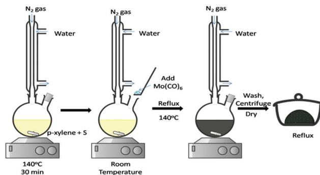
Fig. 8 Reaction between Mo(CO)<sub>6</sub> and S under a nitrogen atmosphere to synthesise MoS<sub>2</sub> NPs.<sup>65</sup>
