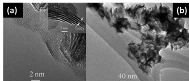
Fig. 5 HRTEM image of MoSe<sub>2</sub> prepared by a hydrothermal method. Reprinted with permission from ref. 52 [H. Tang, K. Dou, C.-C. Kaun, Q. Kuang and S. Yang, *J. Mater. Chem. A*, 2014, **2**, 360–364]. Copyright The Royal Society of Chemistry.
