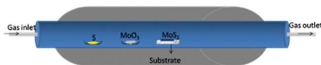
Fig. 10 Experimental setup for the reaction carried out in a tube furnace.<sup>80</sup>
