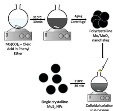
Fig. 9 Synthesis of ultra-small MoS<sub>2</sub> NPs using oleic acid.<sup>66</sup>
