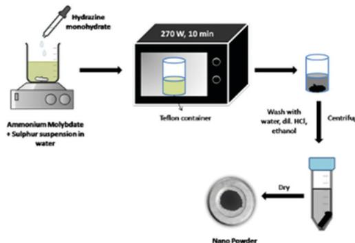
Fig. 15 Microwave synthesis of rod-shaped  $\text{MoS}_2$  NPs.<sup>107</sup>
