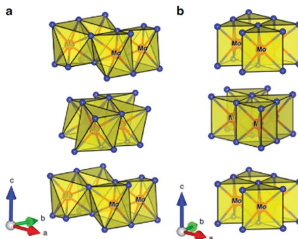
Fig. 3 Crystal structure of (a) monoclinic 1T'-MoTe<sub>2</sub> and (b) hexagonal 2H-MoTe<sub>2</sub> phases. Reprinted with permission from ref. 28 [J. C. McGlynn, T. Dankwort, L. Kienle, N. A. G. Bandeira, J. P. Fraser, E. K. Gibson, I. Cascallana-Matias, K. Kamaras, M. D. Symes, H. N. Miras and A. Y. Ganin, *Nat. Commun.*, 2019, **10**, 4916]. Copyright 2019, The Authors.
