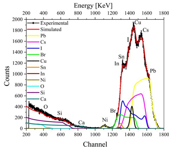
Fig. 4 RBS spectrum of the complete device excited from the Cu contact side, with simulation and deconvolution of the elemental spectra for glass/ITO/ $\text{NiO}_x$ /CsPbI<sub>2</sub>Br/C<sub>60</sub>/Cu.
