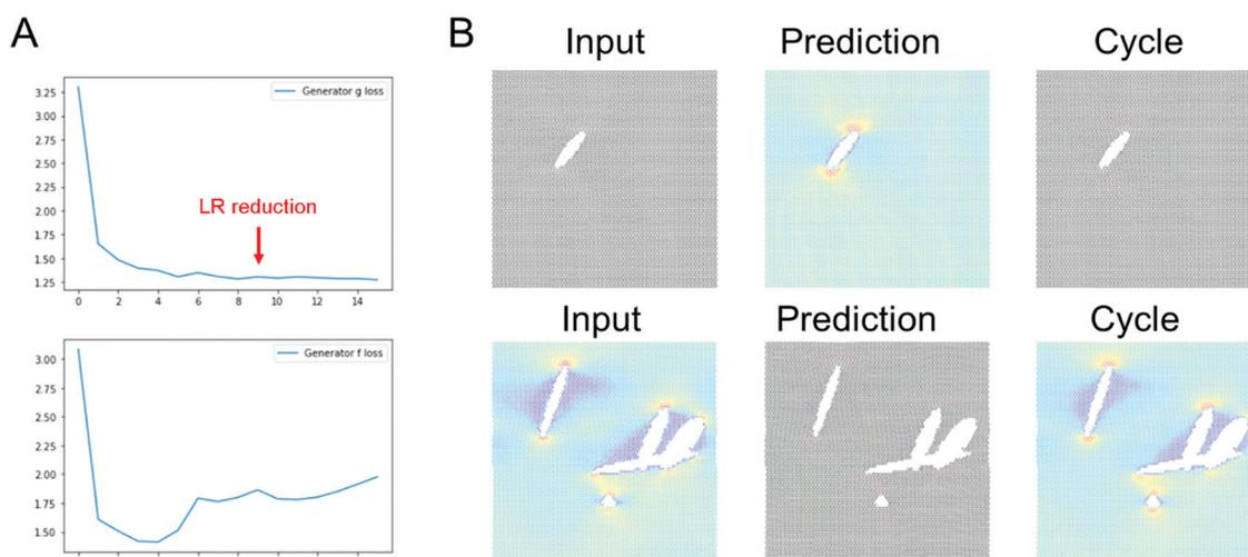
**Fig. 4** Results using the U-Net architecture. Panel A shows the generator loss and discriminator loss functions, respectively. Panel B depicts a few sample results, for two distinct inputs (top: microstructure, bottom: stress field). The cycle prediction, comparing to the input, indicates that cycle consistency has been achieved. Note, as shown in Panel A, we reduce the learning rate from  $2 \times 10^{-4}$  to  $2.5 \times 10^{-5}$  after 9 epochs.
