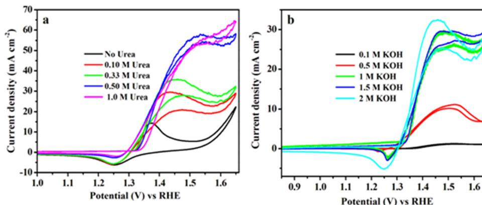
Fig. 8 CV responses of 35-Ni-ttc-d/g-C<sub>3</sub>N<sub>4</sub> at a scan rate of 50 mV s<sup>-1</sup> (a) with variable urea concentrations in fixed 1 M KOH solution saturated with N<sub>2</sub> and (b) with different KOH concentrations in fixed 0.33 M urea solution saturated with N<sub>2</sub>.
