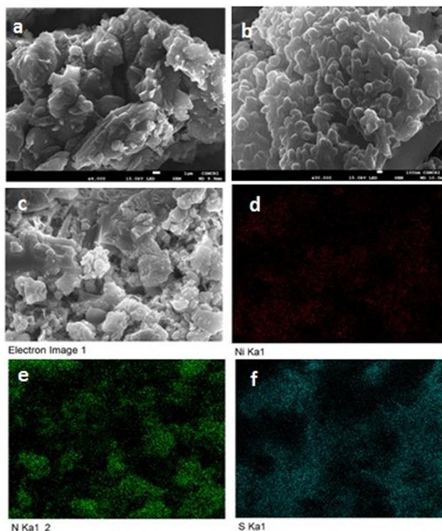
Fig. 4 (a and b) FESEM images of g-C<sub>3</sub>N<sub>4</sub> and 35-Ni-ttc-d/g-C<sub>3</sub>N<sub>4</sub>, respectively, and (c–f) SEM-EDX elemental mapping of 35-Ni-ttc-d/g-C<sub>3</sub>N<sub>4</sub>.
