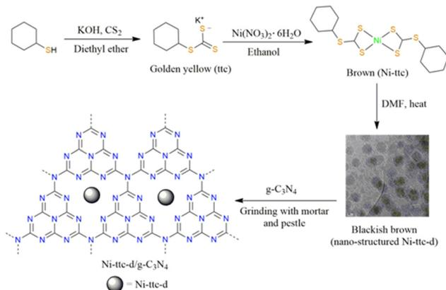
Scheme 1 Preparation of Ni-ttc, Ni-ttc-d, and Ni-ttc-d/g-C<sub>3</sub>N<sub>4</sub>.
