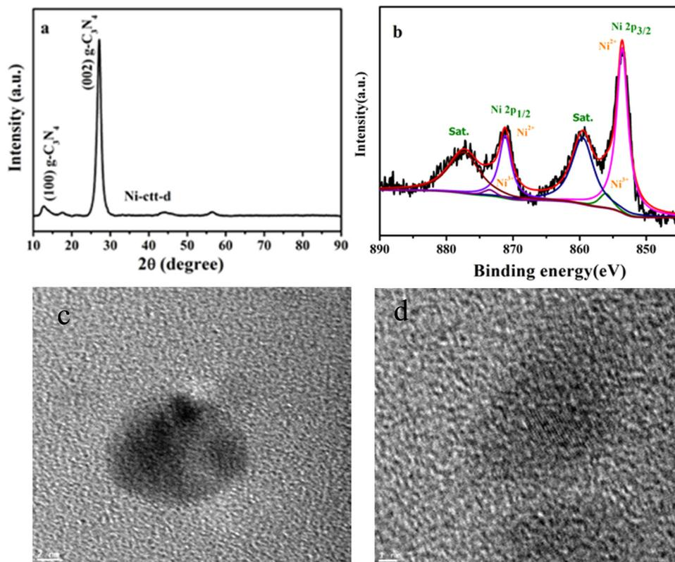
Fig. 10 (a) Powder XRD patterns of 35-Ni-ttc-d/g-C<sub>3</sub>N<sub>4</sub> after the long-term UOR. (b) The Ni 2p XPS spectra of 35-Ni-ttc-d/g-C<sub>3</sub>N<sub>4</sub> after the long-term UOR. (c and d) HRTEM images of 35-Ni-ttc-d/g-C<sub>3</sub>N<sub>4</sub> after the long-term UOR.
