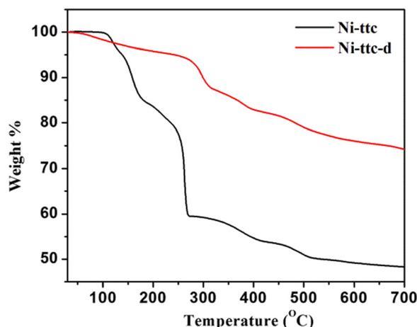
Fig. 6 TGA curves of Ni-ttc and Ni-ttc-d.
