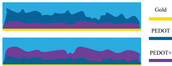
Fig. 6 Stacked polymerization of PEDOT and PEDOT+ on top of gold in aqueous solution. Layers top to bottom (top) PEDOT, PEDOT+, and gold and (bottom) PEDOT+, PEDOT, and gold with the respective PEDOT and PEDOT+ becoming the dominant top layer.
