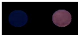
Fig. 4 Image of rGO-D TPP -coated paper strip sensor (left) and strip treated with F^- ions (right) under 365 nm UV light illumination.
