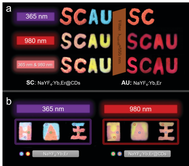
Fig. 4 (a) The photographs of “SCAU” patterns made with NaYF 4 :Yb,Er@CDs and NaYF 4 :Yb,Er under 365 nm, 980 nm, and 365 nm & 980 nm irradiation for dual-mode anti-counterfeiting. (b) The photographs of graphic security patterns made with NaYF 4 :Yb,Er and NaYF 4 :Yb,Er@CDs under 365 nm and 980 nm irradiation for dual-mode anti-counterfeiting.
