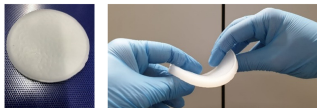
Fig. 8 Paraffin gelator/polyolefin composite before and after melting.
