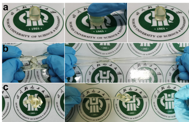
Fig. 3 The poly(AM-co-AA)/GQD hydrogels (1 wt% GQDs) exhibited significant mechanical toughness ((a) compressed and released, (b) cross-bent and stretched, and (c) knotted and stretched).
