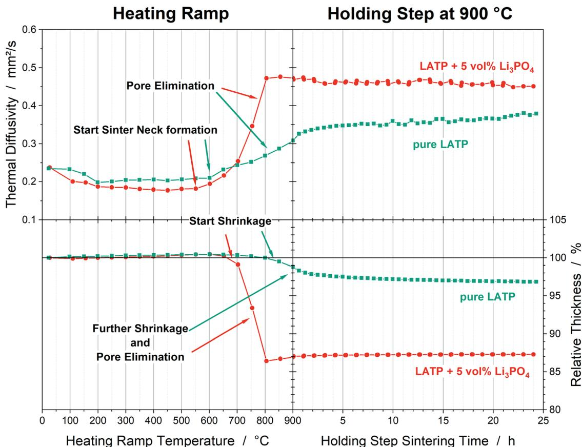
Fig. 3 Thermal diffusivities and relative densities of the pure LATP (green) and LATP + 5 vol%  $\text{Li}_3\text{PO}_4$  (red) pellets sintered at 900 °C. The heating ramp is plotted as a function of temperature; the holding step is plotted as a function of time. The trends during the heating ramp are representative of all pellets of the same composition (Fig. S2, ESI†).
