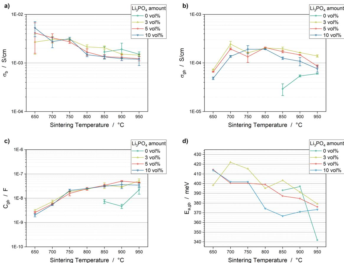
Fig. 7 Electrical properties as a function of the sintering temperature: (a) bulk conductivity,  $\sigma_b$ ; (b) grain boundary conductivity,  $\sigma_{gb}$ ; (c) grain boundary capacitance,  $C_{gb}$ ; (d) grain boundary activation energy,  $E_{a,gb}$ .
