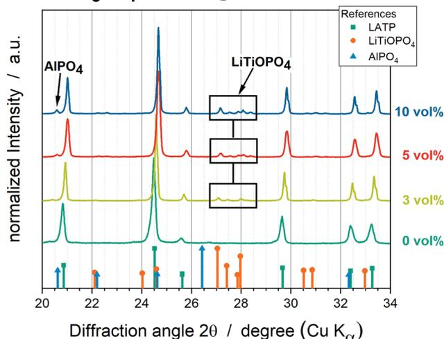
Fig. 1 XRD patterns of all powder mixtures sintered at 900 °C. Pure LAMP (dark green), LAMP + 3 vol% Li<sub>3</sub>PO<sub>4</sub> (light green), LAMP + 5 vol% Li<sub>3</sub>PO<sub>4</sub> (red) and LAMP + 10 vol% Li<sub>3</sub>PO<sub>4</sub> (blue).
