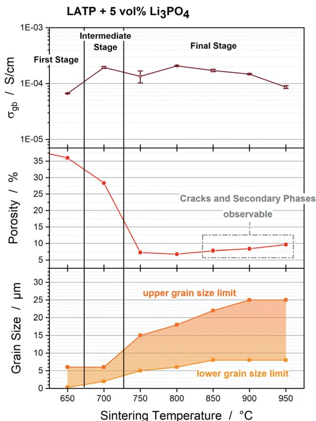
Fig. 8 Comparison of the electrochemical and microstructural results of the LTP + 5 vol%  $\text{Li}_3\text{PO}_4$  samples as a function of the sintering temperature: grain boundary conductivity (EIS), porosity (Archimedes principle), grain size and observable crack formation (SEM).
