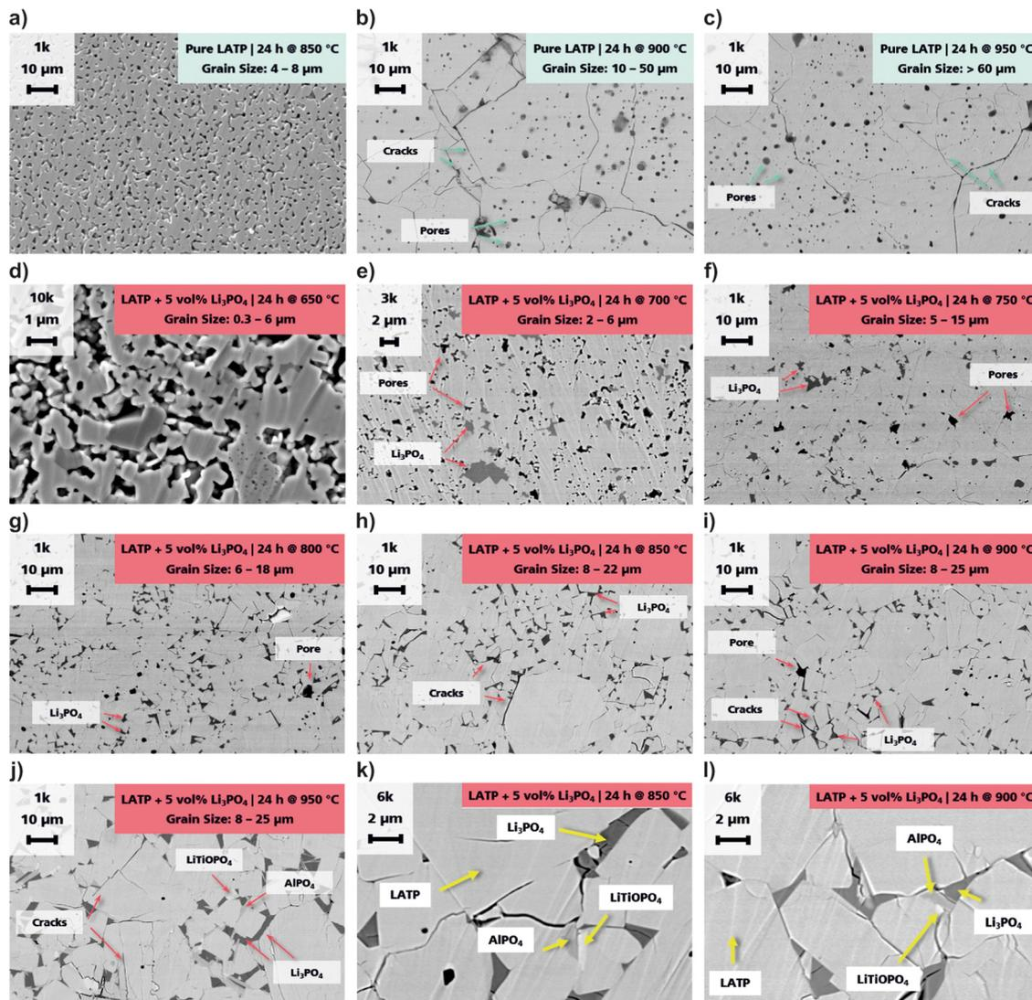
Fig. 5 SEM cross sections of the pure LATP samples sintered at (a) 850 °C, (b) 900 °C and (c) 950 °C and LATP + 5 vol%  $\text{Li}_3\text{PO}_4$  samples sintered at (d) 650 °C, (e) 700 °C, (f) 750 °C, (g) 800 °C, (h) and (k) 850 °C, (i) and (l) 900 °C and (j) 950 °C. The sintering time was 24 h. The accelerating voltage was 5 kV. A backscattered electron detector was used to obtain a higher contrast.
