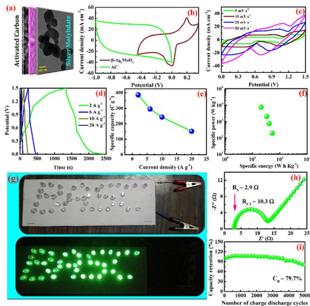
Fig. 6 (a) Schematic representation of BASCs, (b) CV curves of AC (−1 to 0 V) and  $\beta$ - $\text{Ag}_2\text{MoO}_4$  (−0.45 to 0.35 V), supercapacitor performance of cell: (c) CV curves, (d) GCD curves, (e)  $C_S$  vs.  $I_D$ , (f) Ragone plot, (g) charged cell is energizing the green LEDs, (h) Nyquist plot and (i) cyclic stability.
