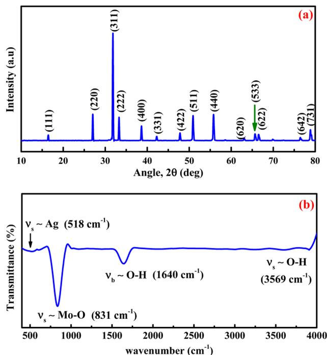
Fig. 1 (a) XRD pattern and (b) FTIR spectrum of β-Ag<sub>2</sub>MoO<sub>4</sub> nanostructures.
