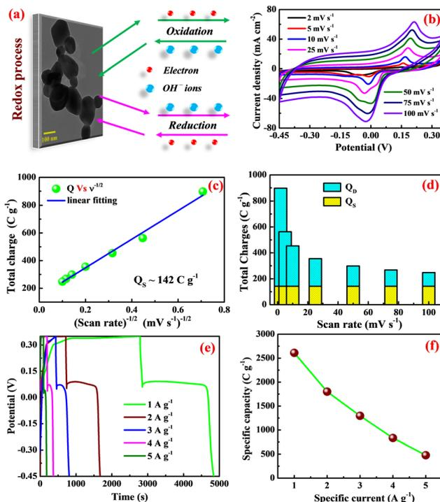
Fig. 4 Electrochemical measurements of  $\beta$ - $\text{Ag}_2\text{MoO}_4$ : (a) redox mechanism, (b) CV curves, (c)  $Q_T$  versus  $\nu^{-1/2}$ , (d) illustration of diffusion/surface charges contribution to total charges stored at various scan rates, (e) GCD curves and (f) capacity versus current.
