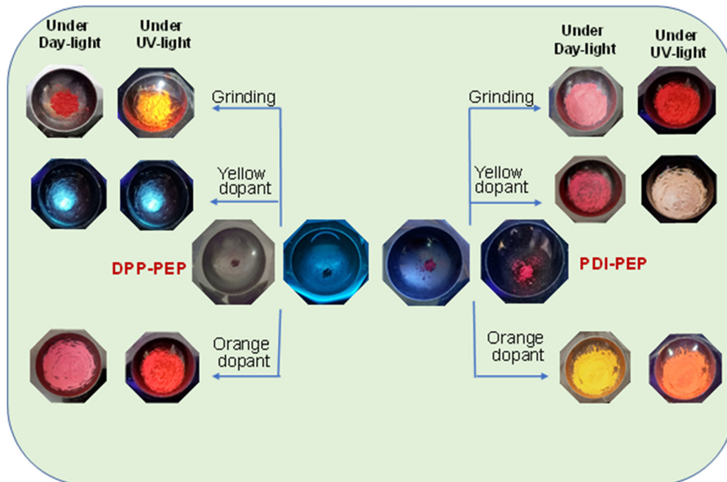
Fig. 5 External stimuli response of the molecules under UV light and daylight of PDI-PEP and DPP-PEP with different dopants.
