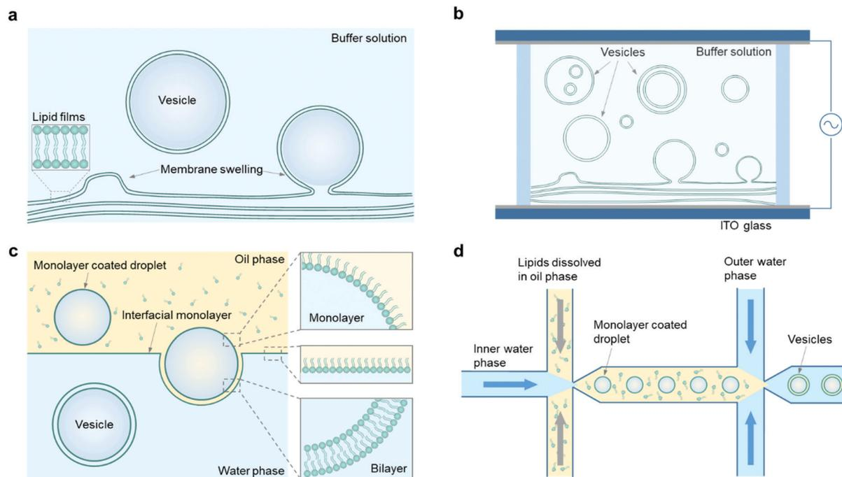
**Fig. 2** Engineering strategies for constructing giant vesicles. (a) Gentle hydration methods. (b) Electro-formation of dry lipid films results in the formation of vesicles. Note that lipid films can be deposited on one or both ITO slides. (c) Vesicles are generated by droplet phase transfer through a lipid-stabilized oil–water interface. (d) Microfluidic generation of w/o/w double emulsions and subsequent oil extraction results in the formation of giant vesicles.
