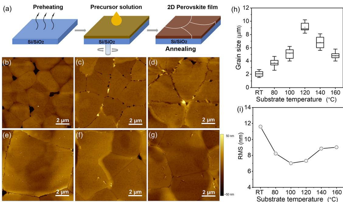
**Fig. 2** (a) Schematic diagram of the hot-casting process. AFM height images of thin (TEA)<sub>2</sub>SnI<sub>4</sub> films processed at the substrate temperature of (b) RT, (c) 80 °C, (d) 100 °C, (e) 120 °C, (f) 140 °C and (g) 160 °C. (h) Grain size and (i) film root mean square roughness as a function of substrate temperature.
