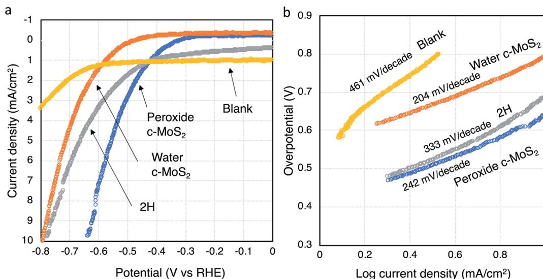
Fig. 6 HER activity of MoS<sub>2</sub> catalysts. (a) Linear sweep voltammograms of all catalysts, normalized by geometric surface area, and (b) corresponding Tafel plots. An uncoated graphite rod ('blank') is used as reference for comparison.
