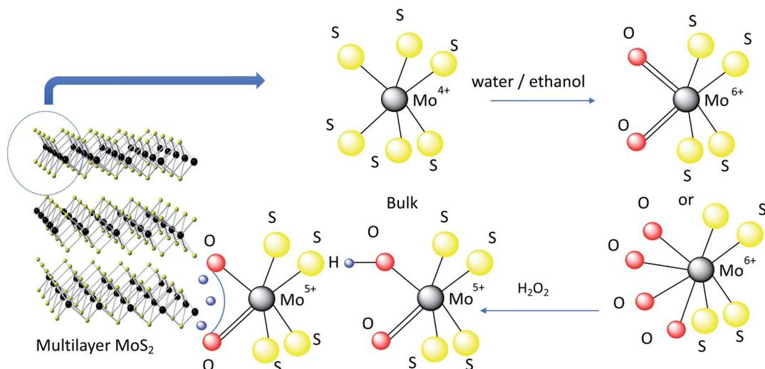
Fig. 5 Schematic representation of the mechanism of formation of conductive  $\text{MoS}_2$ .
