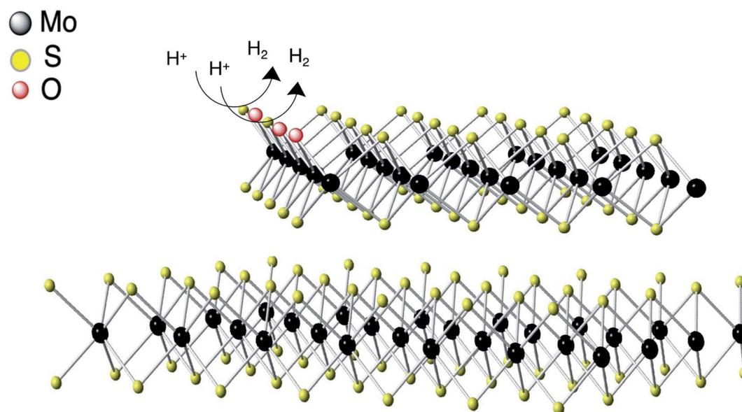
Fig. 7 Schematic representation of HER mechanism of conductive MoS<sub>2</sub>. Hydrogen evolution reaction process at the edges of conductive MoS<sub>2</sub>.
