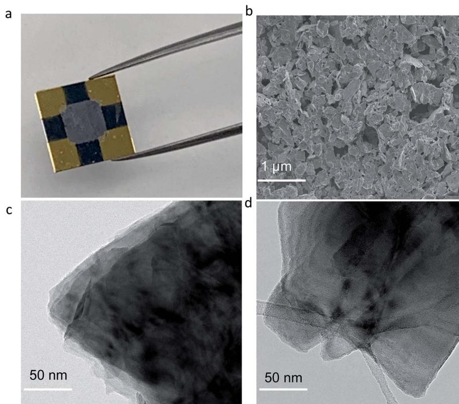
Fig. 2 Surface morphology of MoS<sub>2</sub> samples. (a) Water exfoliated c-MoS<sub>2</sub> (grey area ~7 × 7 mm<sup>2</sup>) on SiO<sub>2</sub> substrate (1 × 1 cm<sup>2</sup>) with Au contacts, and (b) SEM image of water exfoliated c-MoS<sub>2</sub>. The scale bar is 1 μm; (c) TEM image of bulk MoS<sub>2</sub>; and (d) TEM image of water exfoliated conductive MoS<sub>2</sub>. Scale bar for both TEM images is 50 nm.
