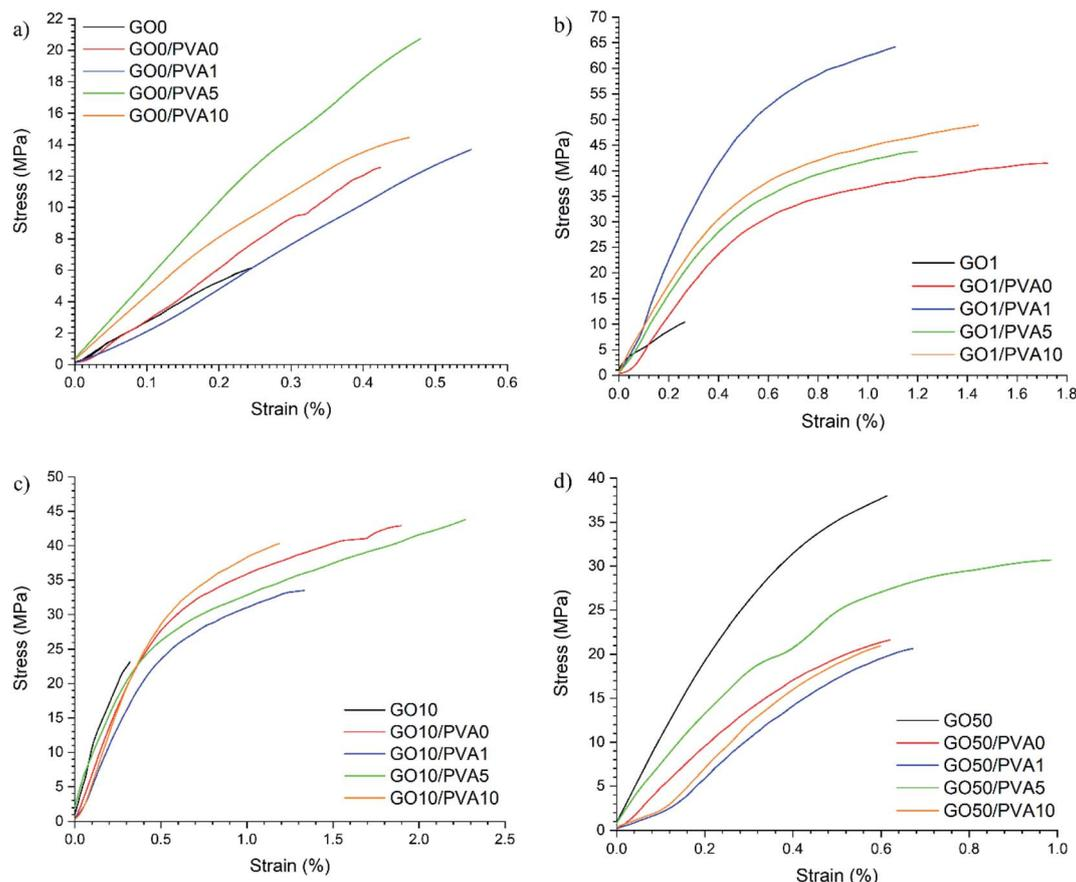
Fig. 5 Representative stress–strain curves for the GO<sub>x</sub>/PVA<sub>y</sub> films where (a) GO<sub>0</sub>, (b) GO<sub>1</sub>, (c) GO<sub>10</sub> and (d) GO<sub>50</sub> based films (the moduli are determined from the steepest part of the slope of the stress–strain curves, within the linear elastic region).
