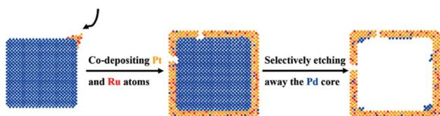
Scheme 1 Schematic illustration of the synthesis of the PdPtRu nanocages, including the co-deposition of Pt and Ru atoms on Pd nanocubes, and the selective removal of the Pd core via chemical etching.
