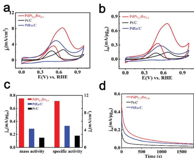
Fig. 2 (a and b) Cyclic voltammograms (CVs) of three different catalysts including PdPt<sub>2.5</sub>Ru<sub>2.4</sub> nanocages (red), commercial Pt/C (black) and commercial PtRu/C (blue) for the MOR normalized by the ECSA and Pt mass, respectively. (c) Specific and mass activity at the peak position of the forward curve. (d) Current–time curves (*I*–*t*) for methanol electrooxidation of these three catalysts at the peak position voltage (vs. RHE) for 1800 s.
