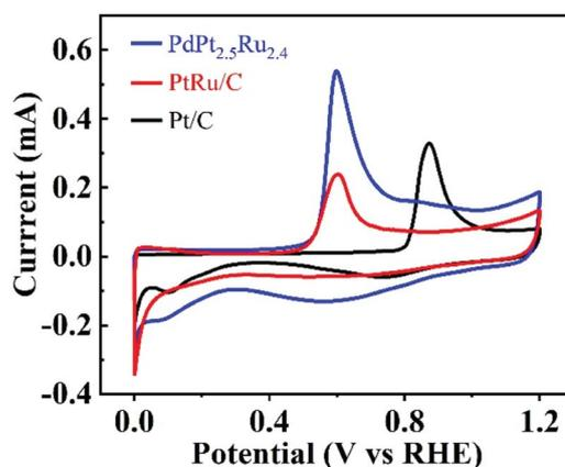
Fig. 3 CO stripping voltammograms of three different catalysts including PdPt<sub>2.5</sub>Ru<sub>2.4</sub> nanocages (red), commercial Pt/C (black) and commercial PtRu/C (blue) recorded in 0.1 M HClO<sub>4</sub> aqueous solution.
