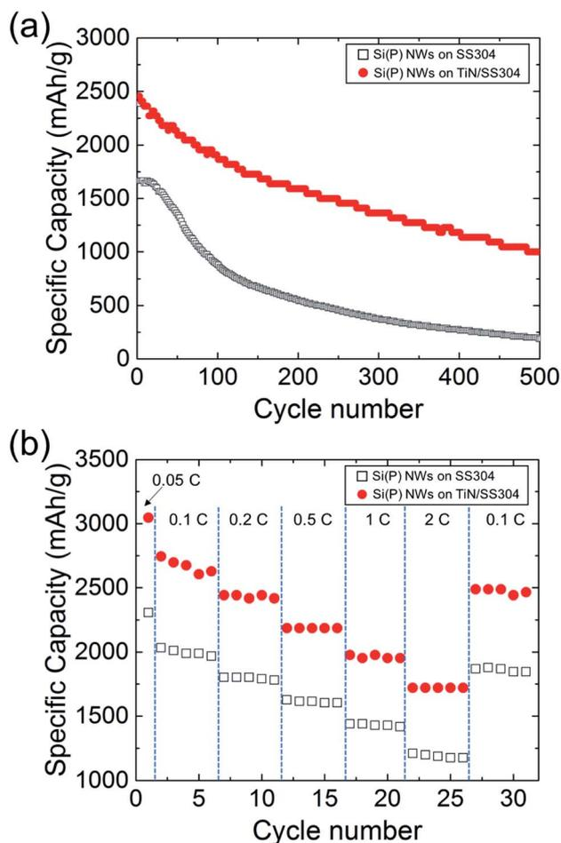
Fig. 5 Specific gravimetric capacities of Si(P) NWs grown on SS304 (black, square, empty) and on TiN/SS304 (red, circle, solid) over cycling at  $800 \text{ mA g}^{-1}$  ( $0.2\text{C}$  for Si) (a) and at different charging rates (b).
