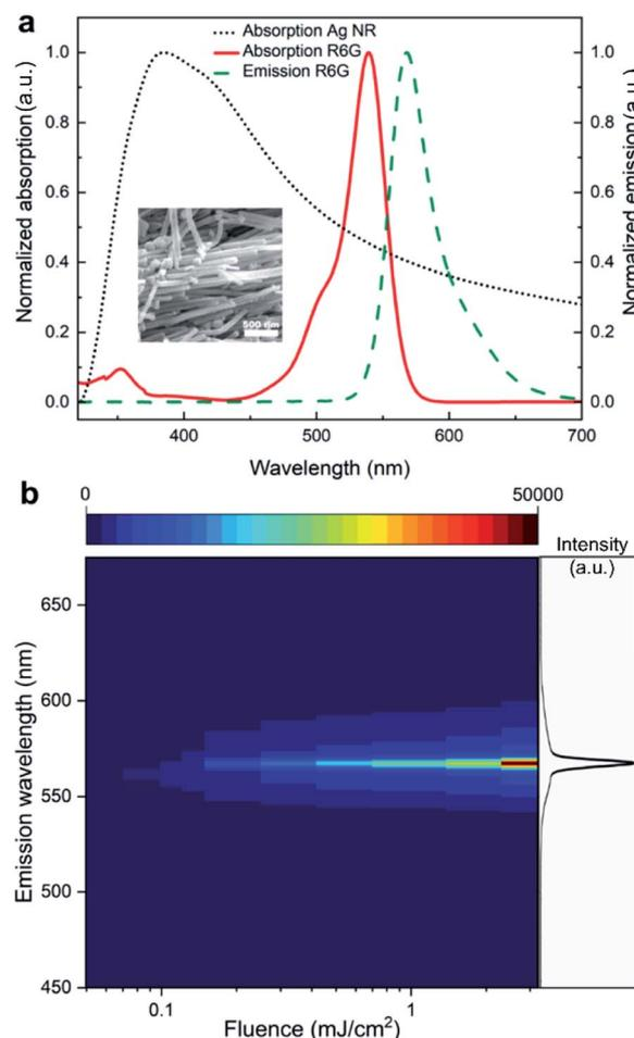
**Fig. 1** (a) Normalised absorption spectra of the silver nanorods and rhodamine 6G and the emission spectrum of rhodamine 6G. Inset shows the SEM image of the silver nanorods. Scale bar represents 500 nm. (b) The evolution of random lasing emission with increasing pump fluence. The spectral profile of the emission at a pump fluence of  $2.7 \text{ mJ cm}^{-2}$  is shown on the right column.
