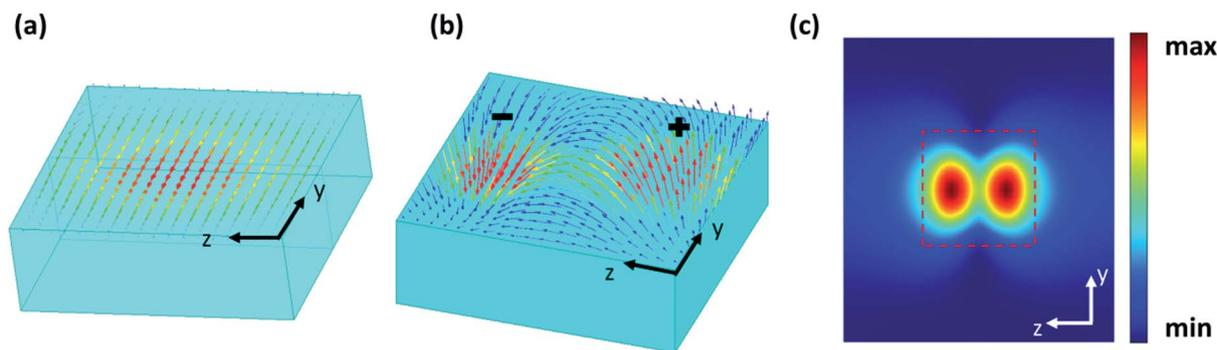
**Fig. 3** (a) The  $yz$ -cross polarization current distribution, (b) the magnetic induction lines excited by the polarization current and (c) the magnetic field of the left silicon particle. The blue cuboids in (a) and (b) are the silicon particles above the gold plate. The red dotted line in (c) represents the silicon particle area.
