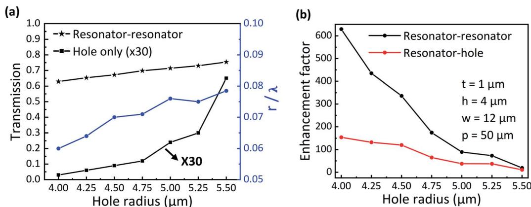
Fig. 6 (a) The black star line shows the peak intensity of the resonator–resonator coupling structure as a function of hole radius. The black square line shows a 30 $\times$  magnification of the transmitted intensity of the hole array structure. The blue circle line shows the variation of  $r/\lambda$  (right axis) with hole radius  $r$ . (b) Enhancement factor as a function of hole radius obtained from resonator–hole coupling (red line) and resonator–resonator coupling (black line) structures.
