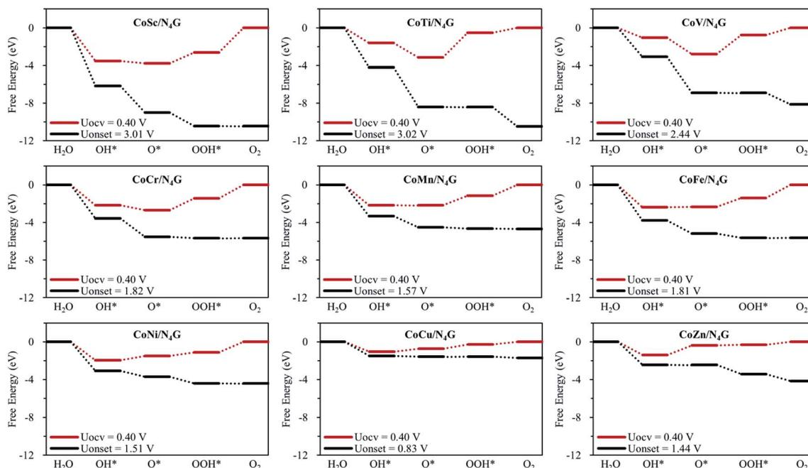
Fig. 3 Free energy diagrams for CoM/N<sub>4</sub>G (M = 3d block metals) at OCV condition ( $U_{\text{OCV}} = 0.401$  V) and onset potential.
