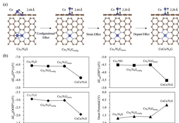
Fig. 5 (a) Decoupled models of the configurational (Co<sub>2</sub>/N<sub>4</sub>G<sub>config</sub>), strain (Co<sub>2</sub>/N<sub>4</sub>G<sub>strain</sub>) and dopant effects. (b) Adsorption energy and onset potential variation of each decoupled model.
