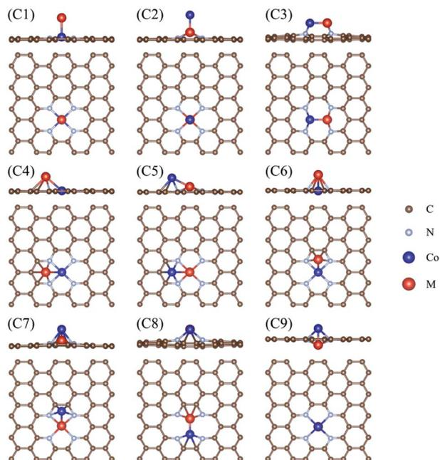
Fig. 2 Types of CoM/N<sub>4</sub>G catalysts considered: (C1) and (C2) have a vertical bonding configuration, and (C3)–(C9) have horizontally or diagonally combined features with a different coordination of N or C atoms.
