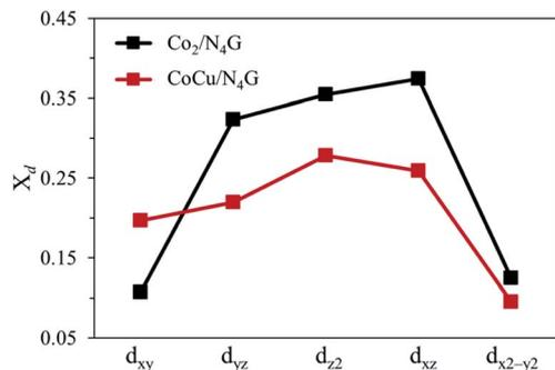
Fig. 7 Overlap ratio ( $X_d$ ) of d-orbitals to p-orbitals. The black dots correspond to the overlap ratio of  $\text{Co}_2/\text{N}_4\text{G}$ , and the red dots are equivalent to the overlap ratio of  $\text{CoCu}/\text{N}_4\text{G}$ .
