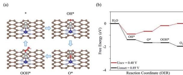
Fig. 9 (a) Schematic diagram of OER on the  $\text{CoPd}/\text{N}_4\text{G}$  catalyst with the most favorable adsorption configuration of each intermediate, (b) the free energy diagram for the OER on the  $\text{CoPd}/\text{N}_4\text{G}$  catalyst at OCV and the onset potential.
