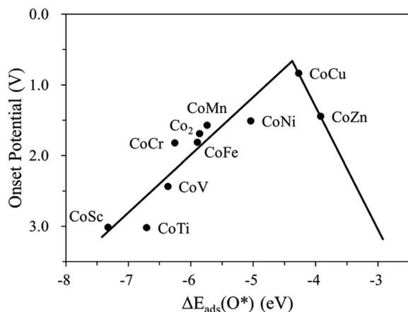
**Fig. 4** Volcano curve indicating the activity (onset potential) for the CoM/N<sub>4</sub>G catalysts (M = 3d block metals) depending on the oxygen adsorption energy,  $\Delta E_{\text{ads}}(\text{O}^*)$ .
