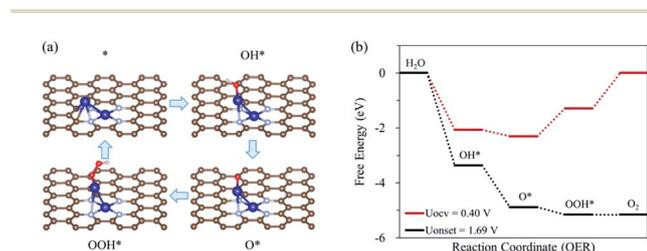
Fig. 1 (a) Schematic diagram of OER on Co<sub>2</sub>/N<sub>4</sub>G catalyst with the most favorable adsorption configuration of each intermediates, (b) free energy diagram depending on the OER pathway on Co<sub>2</sub>/N<sub>4</sub>G at OCV condition ( $U_{\text{OCV}} = 0.401$  V) and onset potential.
