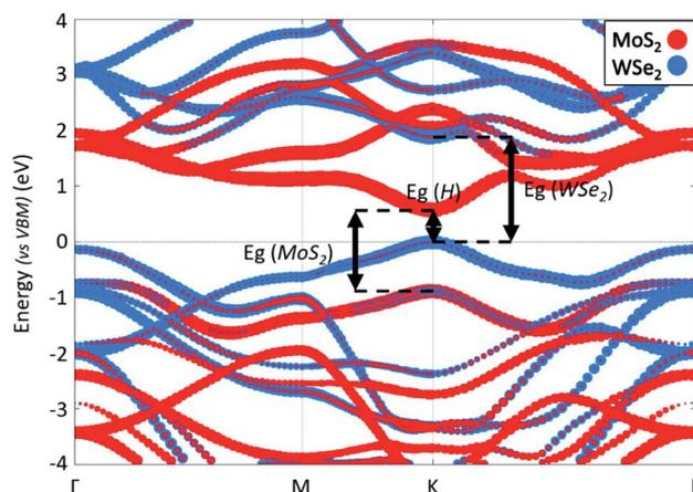
**Fig. 3** Band structure of the MoS<sub>2</sub>/WSe<sub>2</sub> heterojunction along a  $\Gamma$ -M-K- $\Gamma$  path. The energy reference is set to VBM. The red (blue) dots represent electronic states around the nuclei of MoS<sub>2</sub> (WSe<sub>2</sub>).
