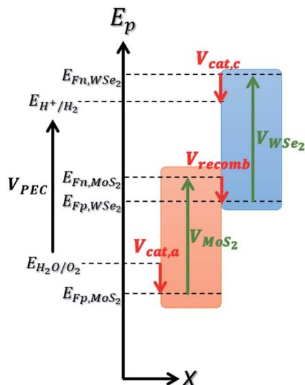
Fig. 2 Representation of the different voltages involved in the computation of  $V_{PEC}$ , depicted on the band diagram of the  $\text{MoS}_2/\text{WSe}_2$  heterojunction. The green arrows represent the voltages generated by the devices. Red arrows represent the losses induced by catalytic overpotentials and carrier's recombination in the region without hBN.  $E_{Fn}$  and  $E_{Fp}$  represent the energy of the pseudo-Fermi level of electrons and holes respectively.
