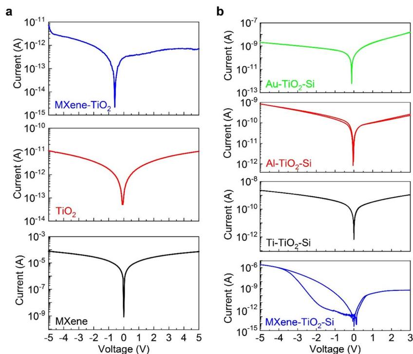
Fig. 2 a)  $I$ – $V$  characteristics of the MXene– $\text{TiO}_2$  junctions,  $\text{TiO}_2$  and MXene films. (b) Performance comparison of the RRAMs with various top-electrodes including Au, Al and Ti and MXene. The resistive area and the performance of MXene– $\text{TiO}_2$ –Si self-rectifying RRAMs, extracted from the  $I$ – $V$  characteristics of 10 devices for each resistive area.
