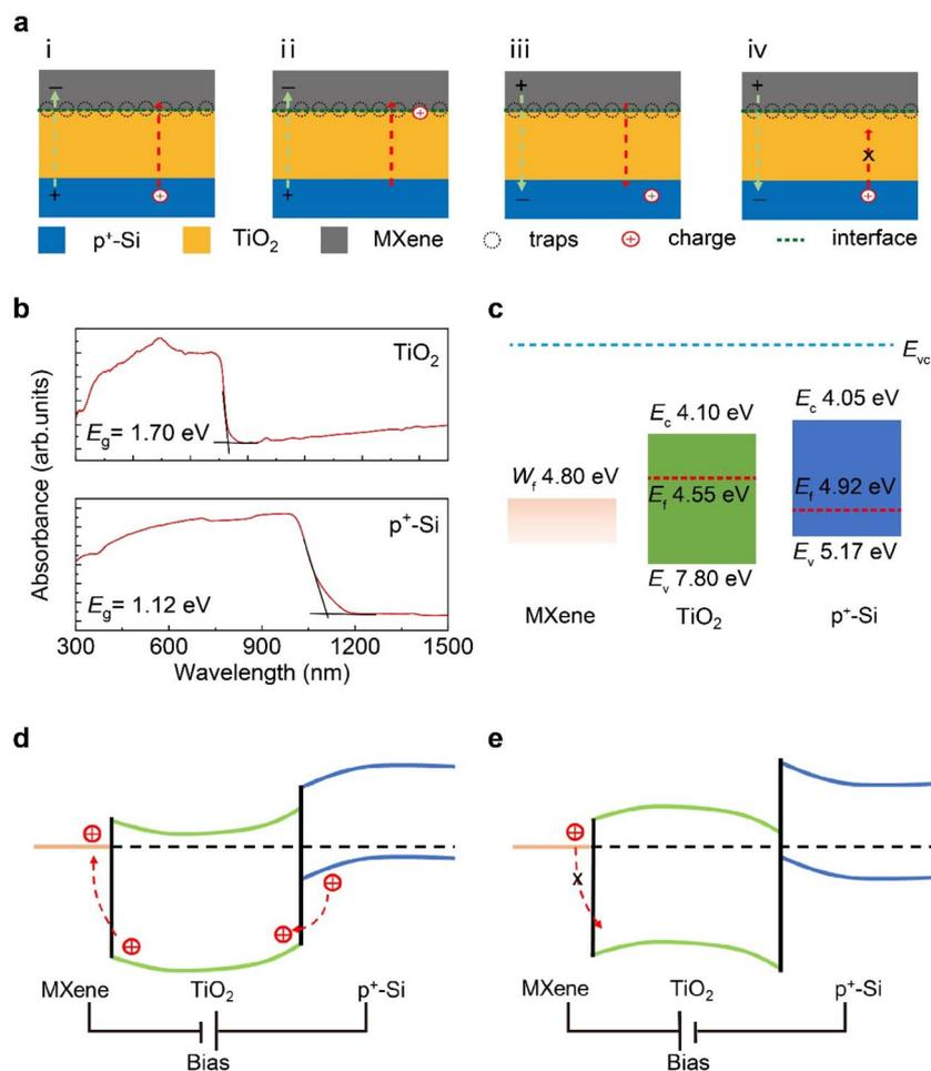
Fig. 4 Mechanism. (a) Resistive switching of the MXene-TiO<sub>2</sub>-Si RRAM device (i.  $V = V_{\text{SET}}$ , ii. Trap, iii. Detrap, iv.  $V = V_{\text{RESET}}$ ). (b) Absorbance spectrum of TiO<sub>2</sub> and p<sup>+</sup>-Si.  $E_g$  is the bandgap. The red line is an auxiliary line for extracting  $E_g$ . (c) Energy band diagram of MXene, TiO<sub>2</sub> and p<sup>+</sup>-Si. Band diagram of the MXene-TiO<sub>2</sub>-Si heterojunction under (d) negative and (e) positive bias.
