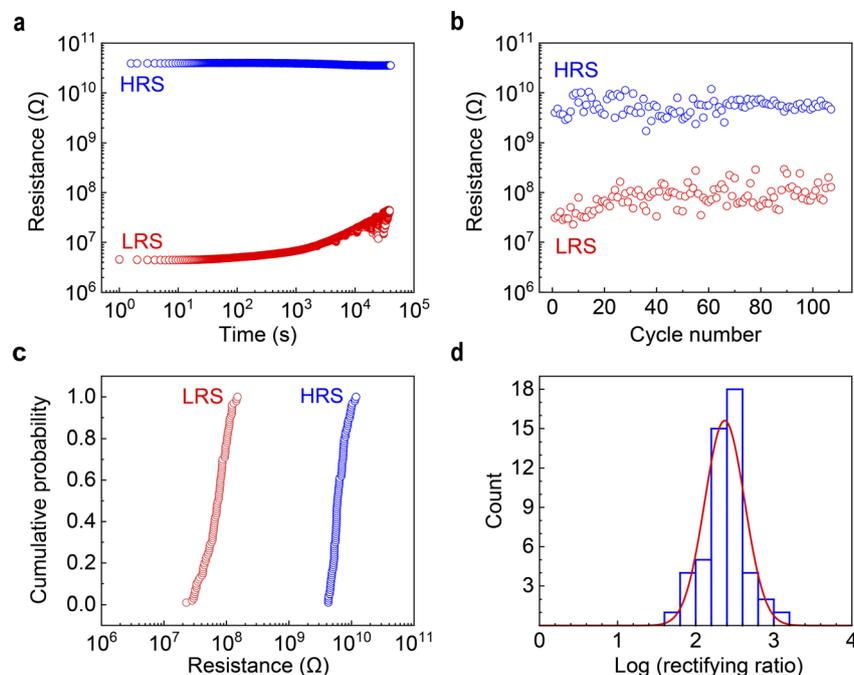
Fig. 3 Evaluation of the electrical performance. (a) Retention and (b) endurance characteristics of the MXene– $\text{TiO}_2$ –Si RRAM obtained at  $\pm 2$  V and the room temperature. (c) Device-to-device cumulative probability of 100 individual MXene– $\text{TiO}_2$ –Si RRAMs based on the resistance of HRS and LRS. (d) Statistical distribution of rectifying ratio of 50 MXene– $\text{TiO}_2$ –Si RRAMs with a standard deviation of 0.25.
