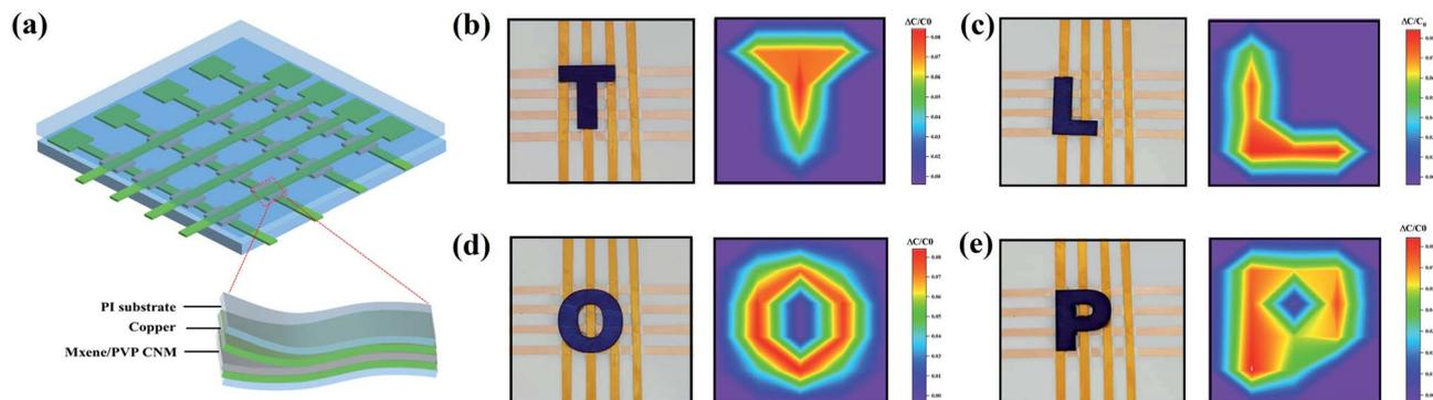
Fig. 5 Spatial pressure distribution based on the sensor array. (a) Schematic diagram of the  $4 \times 4$  sensor array. (b–e) Placement of 3D letters T, L, O and P on the sensor matrix. On the left side there is the actual shape, while on the right there is the capacitance mapping.
