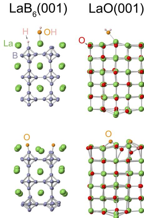
Fig. 3 Snapshots of MD simulations of  $\text{H}_2\text{O}$  adsorption on  $\text{LaB}_6(001)$  (top left) and on  $\text{LaO}(001)$  (top right);  $\text{O}_2$  adsorption on  $\text{LaB}_6(001)$  (bottom left) and on  $\text{LaO}(001)$  (bottom right). O atoms in the  $\text{LaO}$  crystal and those from the adsorbents are denoted by red and orange spheres, respectively.
