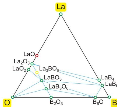
Fig. 1 Calculated ternary phase diagram of the La–B–O system. Green and red circles denote stable and unstable (metastable) compounds, respectively. See the text for the yellow circle (La<sub>3</sub>BO<sub>6</sub>).
