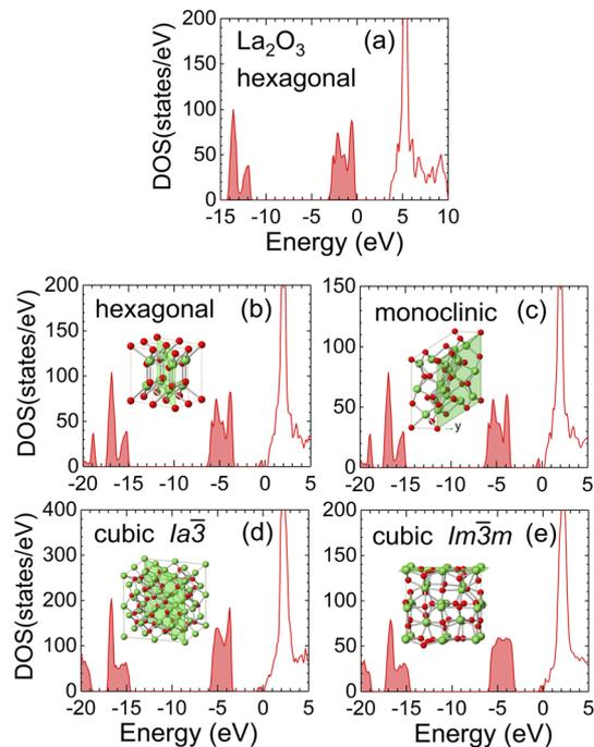
Fig. 4 Electronic DOS of  $\text{La}_2\text{O}_3$  and  $\text{La}_2\text{O}_{3-x}$ . (a) no defects, (b) hexagonal with  $x = 0.125$ , (c) monoclinic with  $x = 0.167$ , (d) cubic ( $Ia\bar{3}$ ) with  $x = 0.125$ , and (e) cubic ( $Im\bar{3}m$ ) with  $x = 0.125$ . The insets depict the surfaces on which the WF was calculated.
