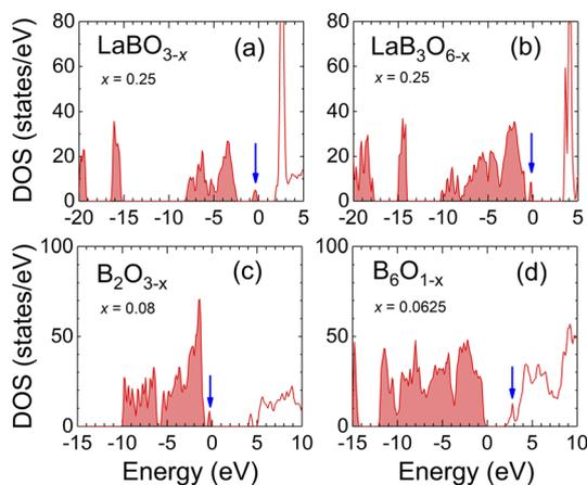
Fig. 5 Electronic DOS of (a)  $\text{LaBO}_{3-x}$ , (b)  $\text{LaB}_3\text{O}_{6-x}$ , (c)  $\text{B}_2\text{O}_{3-x}$ , and (d)  $\text{B}_6\text{O}_{1-x}$ . The blue arrows indicate the defect levels. The Fermi level is set to zero.
