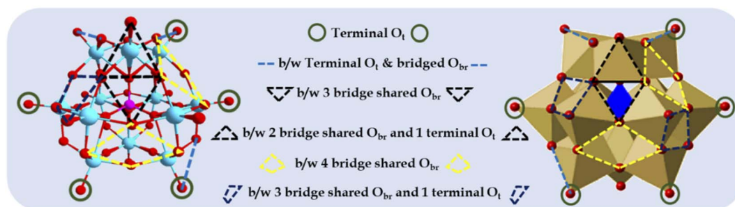
Fig. 1 Different types of surface O atoms and possible anchoring sites for Pd atoms on Keggin-structured anion phosphomolybdic acid.
