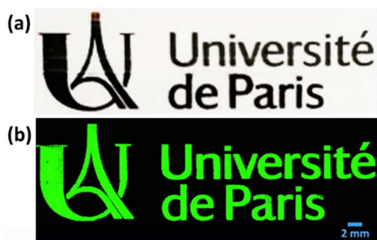
Fig. 7 (a) Inkjet printing pattern of Ag@CCH ink (optical image) and (b) corresponding Raman image recorded by Raman microscope.
