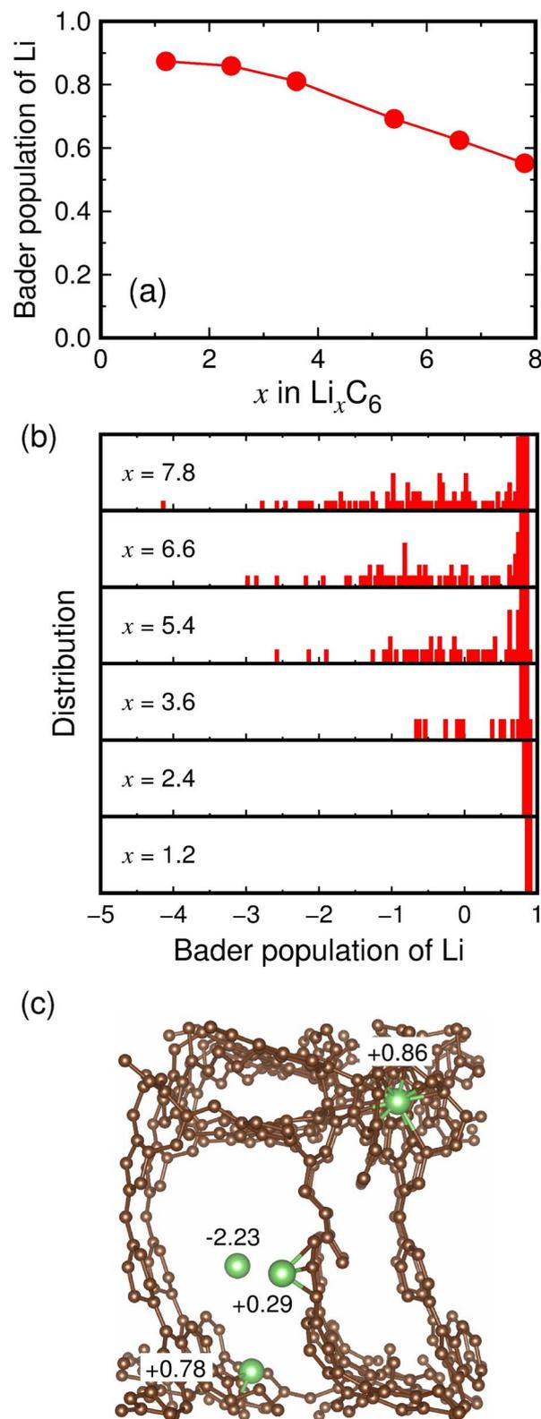
Fig. 5 (a) Average Bader populations of Li and (b) distribution histograms of the Bader populations of Li in lithiated MC-20 structures. (c) Fully lithiated MC-20 ( $Li_{7.8}C_6$ ) structure. All Li atoms are hidden, except for four Li atoms shown to present their charge states.
