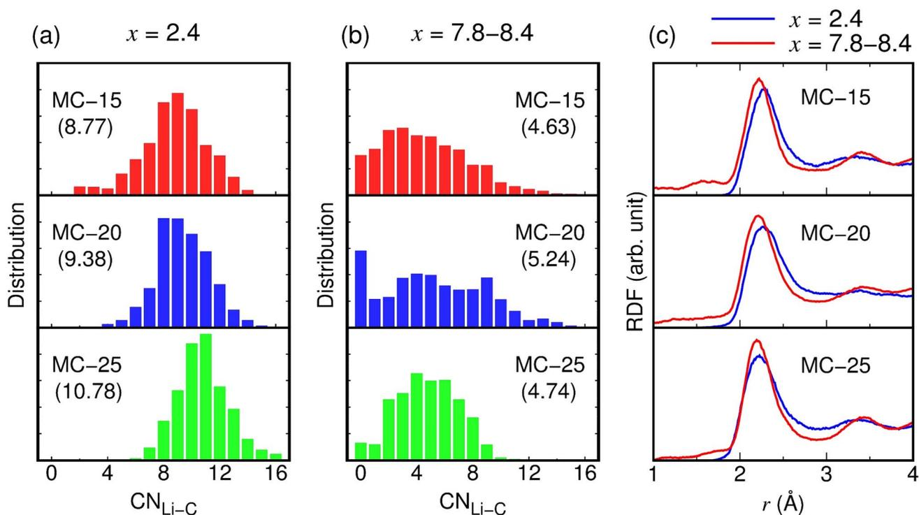
Fig. 7 Structural properties of lithiated microporous carbon structures. Distribution histograms of CN<sub>Li-C</sub> at (a) *x* = 2.4 and (b) *x* = 7.8–8.4. CN<sub>α-β</sub> represents the number of β atoms around an α atom. The atomic bond is connected when the Li–C distance is within 2.9 Å. Values in parentheses indicate the average CN<sub>Li-C</sub>. (c) RDFs of the Li–C pair.
