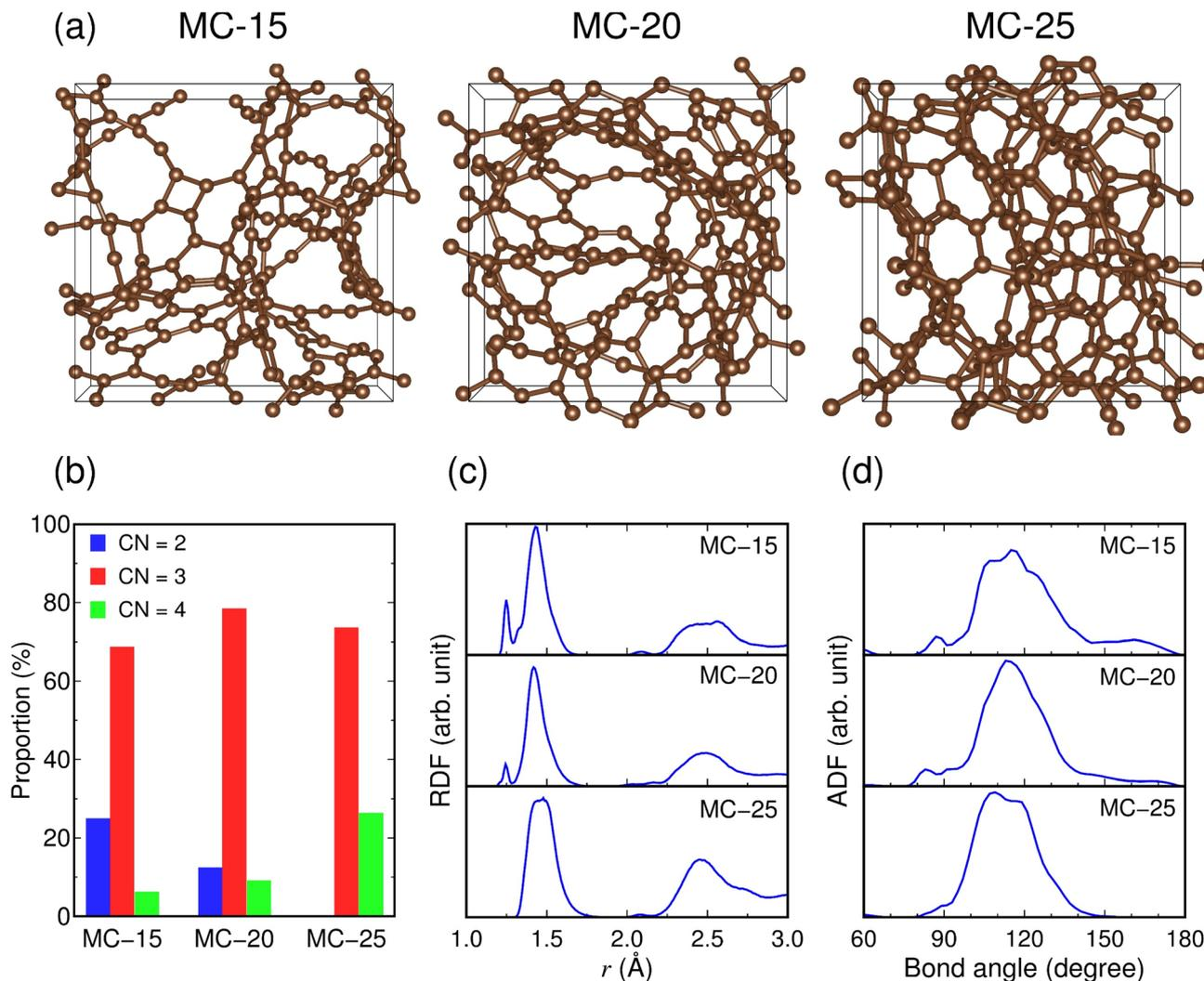
**Fig. 1** (a) Atomic structures and (b–d) structural properties of microporous carbon: (b) proportions of the coordination numbers (CNs) of carbon atoms, (c) radial distribution functions (RDFs) of the C–C pair, and (d) angle distribution functions (ADFs) of the C–C–C bond. The atomic bond is connected when the C–C distance is within 1.9 Å.
