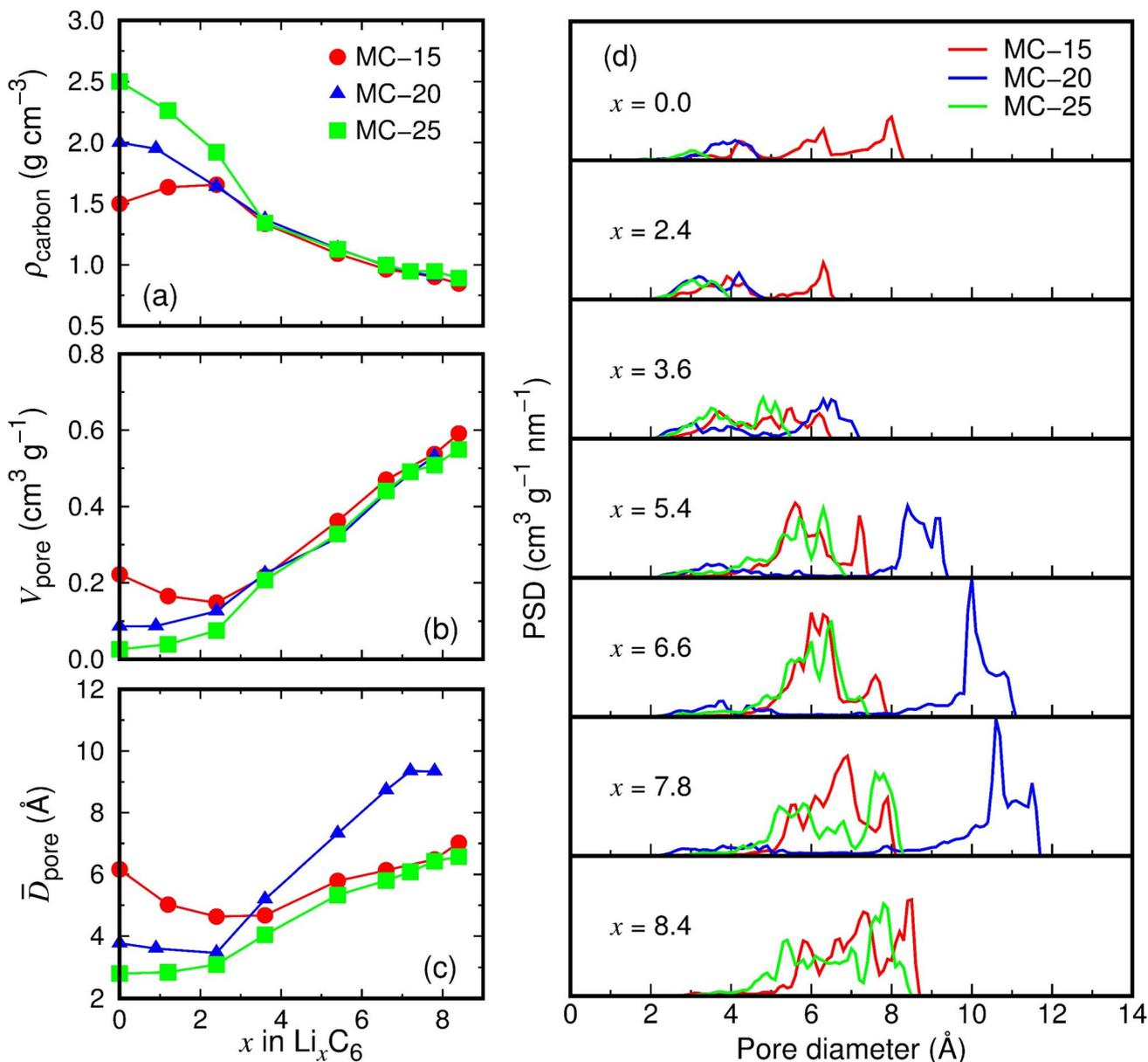
Fig. 4 Structural properties of lithiated microporous carbon structures with Li atoms removed: (a) carbon densities ( $\rho_{\text{carbon}}$ ), (b) total pore volumes ( $V_{\text{pore}}$ ), (c) average pore diameters ( $\bar{D}_{\text{pore}}$ ), and (d) pore size distributions (PSDs).
