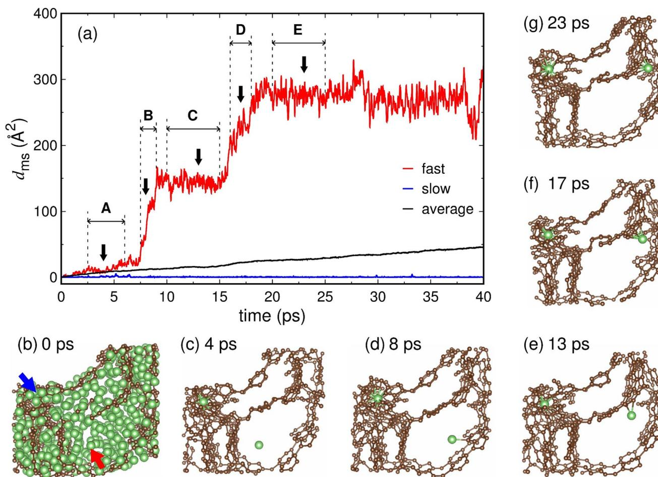
Fig. 8 (a) Mean-square displacements ( $d_{\text{ms}}$ ) of fast- and slow-moving Li ions in the fully lithiated MC-20 ( $\text{Li}_{7.8}\text{C}_6$ ) structure at  $T = 900$  K. Atomic structures at (b) 0, (c) 4, (d) 8, (e) 13, (f) 17, and (g) 23 ps indicated by arrows in (a). In (b), the fast and slow Li ions are indicated by red and blue arrows, respectively. In (c–g), only the two Li ions, indicated by arrows in (b), are shown for clarity of illustration.
