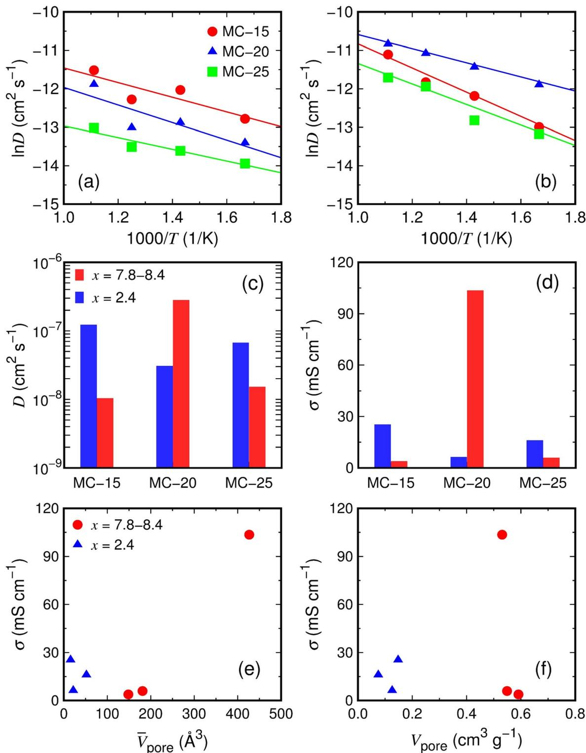
Fig. 6 Diffusion properties of lithiated microporous carbon structures. Logarithmic diffusivities ( $\ln D$ ) of Li ions as a function of inverse temperature at (a)  $x = 1.2$  and (b)  $x = 7.8-8.4$ . (c) Diffusivities ( $D$ ) and (d) conductivities ( $\sigma$ ) of Li ions at  $T = 300 \text{ K}$ . Conductivities of Li ions as a function of (e) average pore volume ( $\bar{V}_{\text{pore}}$ ) and (f) total pore volume ( $V_{\text{pore}}$ ).
