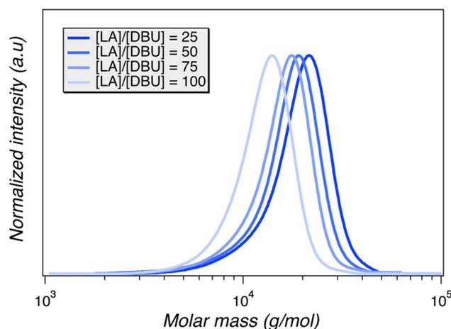
**Fig. 3** SEC chromatograms corresponding to the samples of PLA using various concentrations of DBU catalyst per plug. All samples were generated at fixed flow settings deemed optimal following the flow profile analysis ( $1 \text{ mL min}^{-1}$ ;  $0.6 \text{ Hz}$ ;  $0.04 \text{ mL per stroke}$ ).
