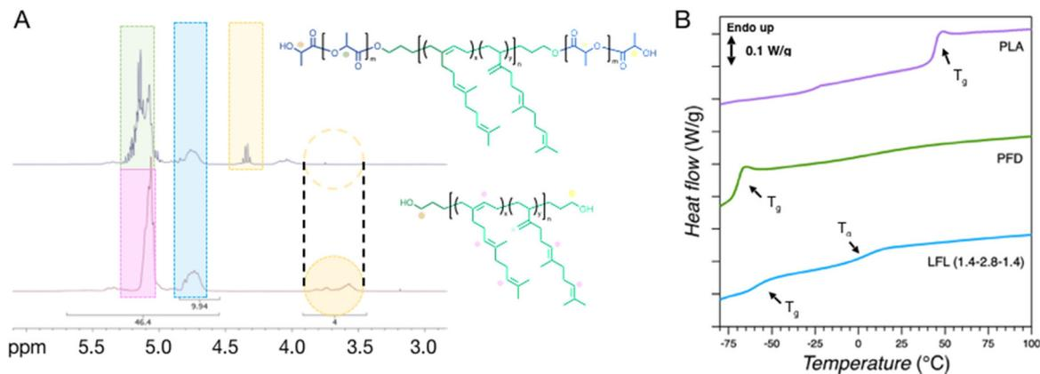
**Fig. 5** (A)  $^1\text{H}$  NMR analysis comparing commercial PFD and the LFL triblock copolymer. (B) DSC analysis of the synthesized LFL triblock copolymer, as well as PLA and the commercial PFD. Characteristic  $T_g$ s are labelled for each sample.
