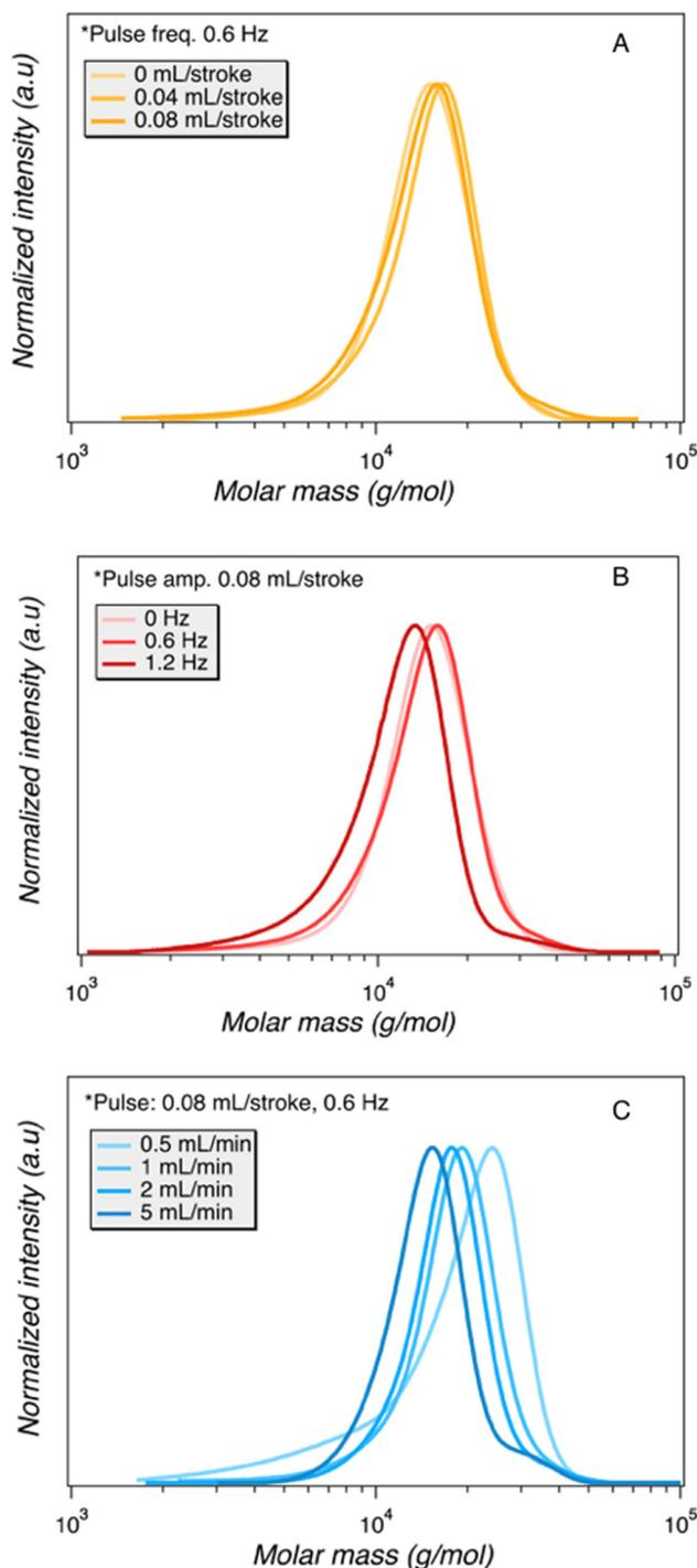
**Fig. 2** Summary SEC chromatograms of different individual parameter variation on molecular weight and distributions. (A) The effect of pulsation amplitude. (B) The effect of pulsation frequency. (C) The effect of flowrate. All polymers had a target molar mass of  $14.4 \text{ kg mol}^{-1}$ .
