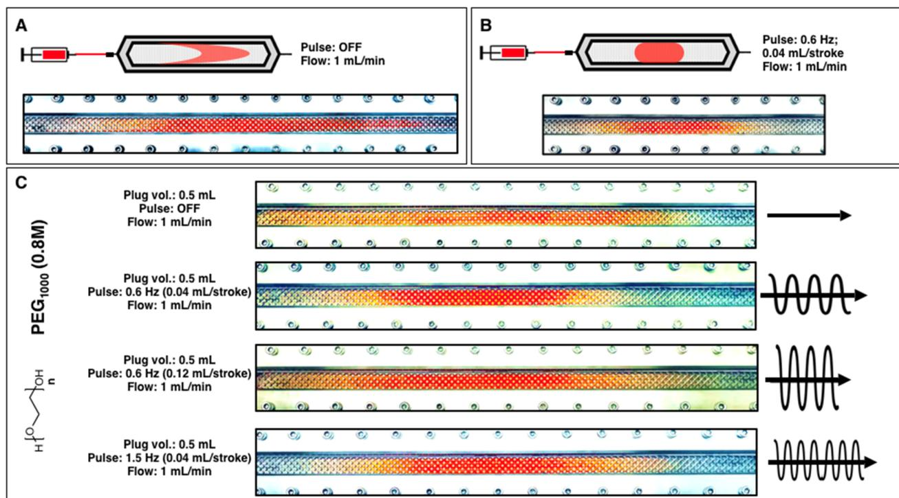
**Fig. 1** Photograph of the flow profile using acetone as a medium. (A) A crescent-shaped flow profile is visible as a result of the formation of a lateral velocity gradient within the reactor in the absence of pulsation. (B) A compact flow profile resulting from pulsation leads to a more homogeneous distribution of the medium in both the longitudinal and lateral direction. (C) A comparison of higher viscosity flow profiles with respect to increasing pulsation frequency and -amplitude.
