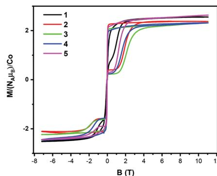
Fig. 15 Pulse-field magnetization curves per cobalt atom for **1–5** at 0.4 K and a sweep rate of 4.10 T ms<sup>-1</sup>.
