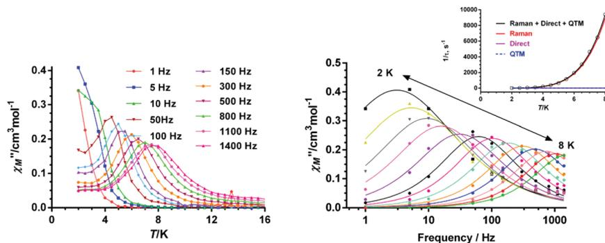
Fig. 12 Temperature dependence of  $\chi''_M$  at different frequencies (left) and frequency dependence at different temperatures (right) for **2** under a field of 0.2 T. Contribution of each relaxation process to the slow relaxation of the magnetization (inset).
