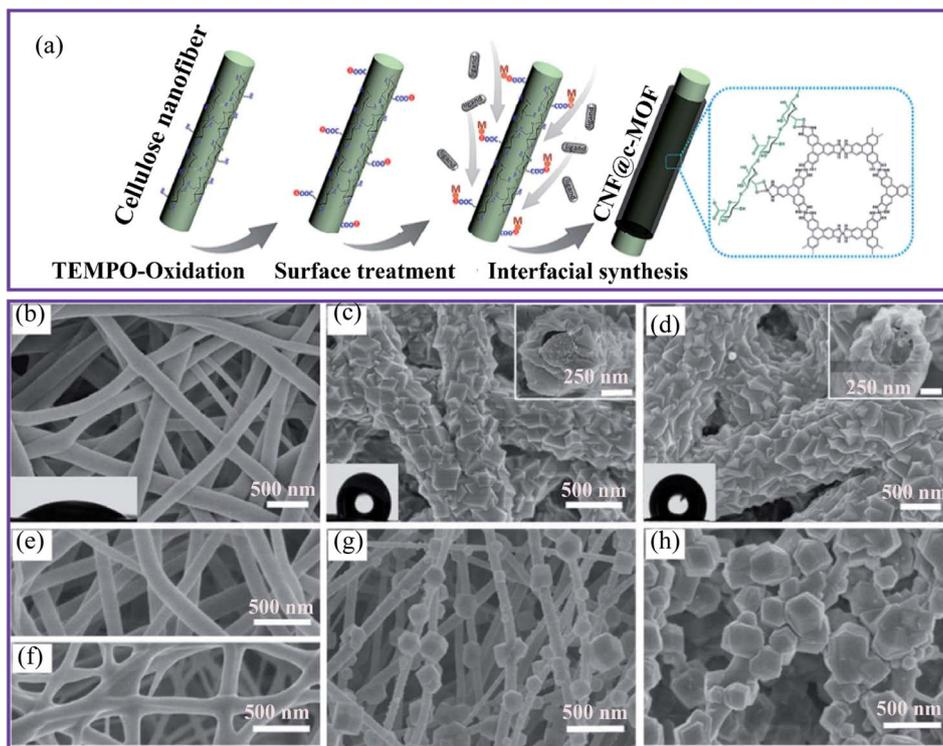
Fig. 2 (a) Schematic diagram of the synthesis of CNF@c-MOF nanofibers.<sup>65</sup> SEM images of (b) the electrospun silk nanofibers, (c) ZIF-8/nanofibers, the inset shows the sectional view from the top, (d) ZIF-67/nanofibers with the sectional view shown in the inset, (e) polyacrylonitrile, (f) polyurethane, (g) PAN@ZIF-8 and (h) PU@ZIF-8 membranes, this figure has been adapted from ref. 36 with permission from the Royal Society of Chemistry, copyright 2018.
