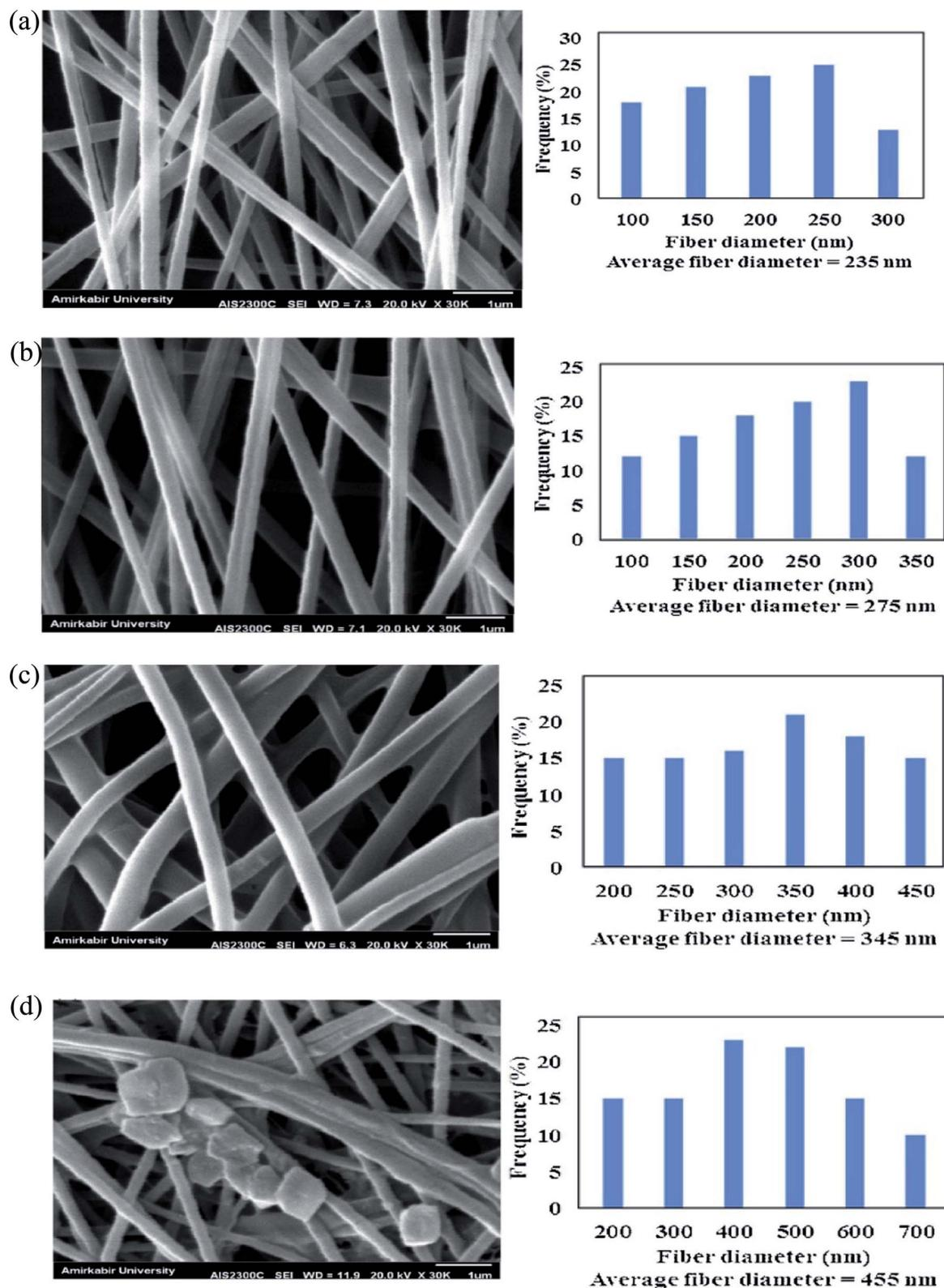
Fig. 5 SEM images and fiber diameter distribution of (a) PAN-chitosan nanofiber and nanofibers containing (b) 5 wt% UiO66-NH<sub>2</sub> MOF, (c) 10 wt% UiO66-NH<sub>2</sub> MOF and (d) 15 wt% UiO66-NH<sub>2</sub> MOF, this figure has been adapted from ref. 74 with permission from Elsevier, copyright 2019.
