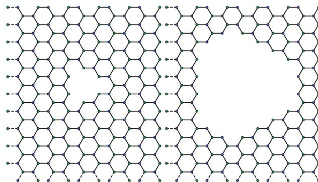
(a) A hole of size 1 — an edge has been removed, as have all edges connected to it. This image represents a network of  $4.72 \text{ nm}$  by  $5.45 \text{ nm}$ . (b) A hole of size 5 — all edges connected to it. This image represents a network of  $4.72 \text{ nm}$  by  $5.45 \text{ nm}$ .
