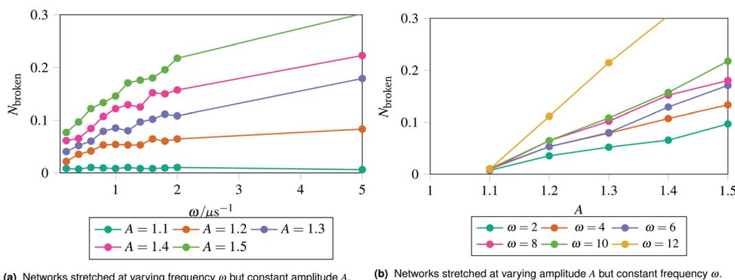
Fig. 5 Recording the fraction of broken bonds at the end of a simulation as a function of stretching frequency  $\omega$  and amplitude  $A$ . The fraction of broken bonds at the end of the simulation increases approximately linearly with both frequency and amplitude, as the most damage is introduced at the maxima and minima of a stretching cycle. The energy inserted into the network at the maxima and minima of stretching is linearly related to the frequency and amplitude.
