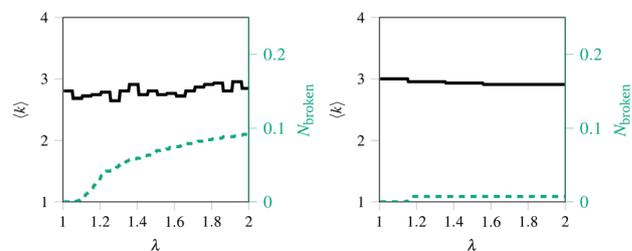
(a) A plot of  $\langle k \rangle$  and  $N_{\text{broken}}$  against  $\lambda$ , (b) A plot of  $\langle k \rangle$  and  $N_{\text{broken}}$  against  $\lambda$ , the stretching ratio for a system with  $D_e = 16.0 \times 10^{-21}$  J and  $\epsilon = 16.0 \times 10^{-21}$  J, the stretching ratio for a system with  $D_e = 128 \times 10^{-21}$  J and  $\epsilon = 128 \times 10^{-21}$  J.
