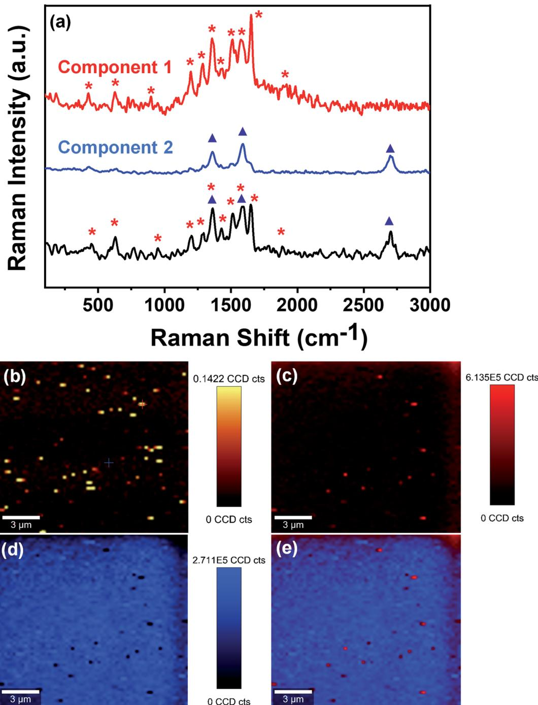
Fig. 10 (a) True component analysis of membrane after filtration, depicting the presence of two components: component 1, *i.e.*, enmeshed contaminant rhodamine B, and component 2 *i.e.*, FMWCNTs, across the color-coded symbols. (b) Large area confocal Raman image, revealing the presence of enmeshed fluorescent rhodamine B (bright spots). (c) Extracted color-coded Raman image of component 1. (d) Extracted color-coded Raman image of component 2. (e) Combined image of components 1 and 2.
