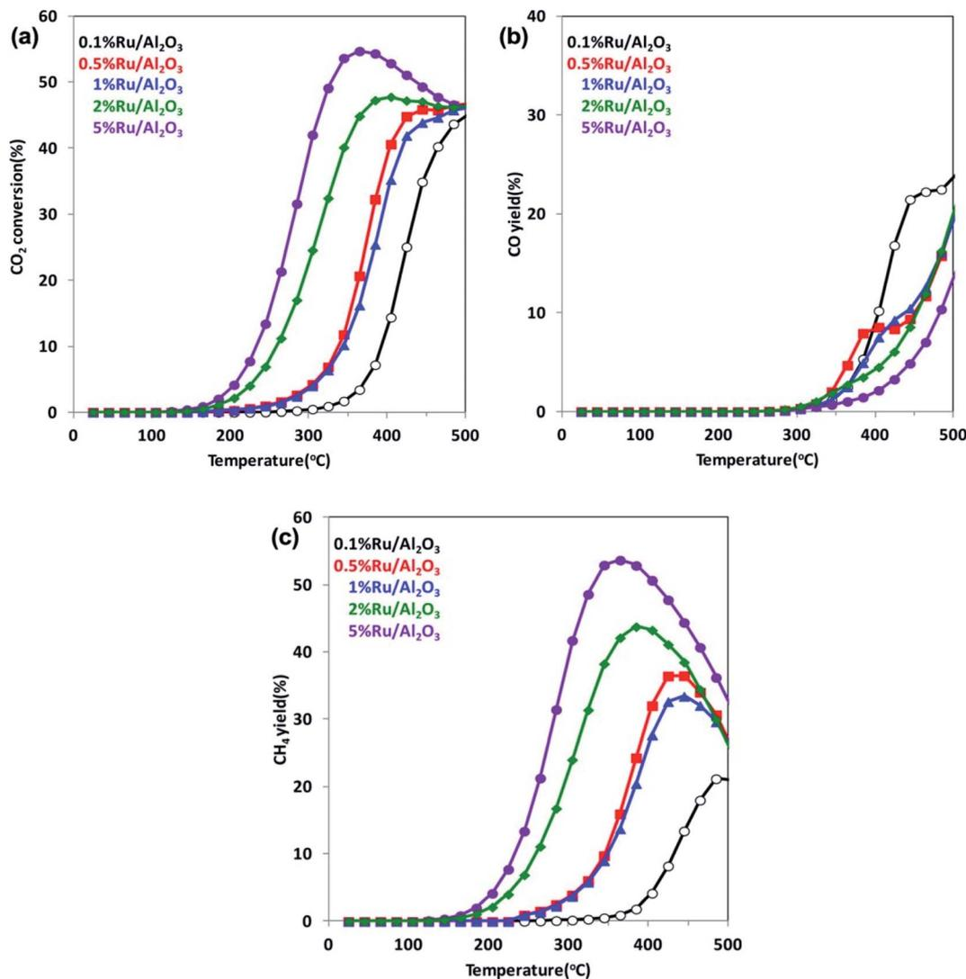
Fig. 6 (a) Temperature dependences of the CO<sub>2</sub> conversion rate over Ru/Al<sub>2</sub>O<sub>3</sub> catalysts for various Ru loadings. (b) and (c) Temperature dependences of the yields of the formation of CO and CH<sub>4</sub>, respectively, over Ru/Al<sub>2</sub>O<sub>3</sub> catalysts for various Ru loadings. Reprinted with permission from ref. 102. Copyright 2013 the American Chemical Society.
