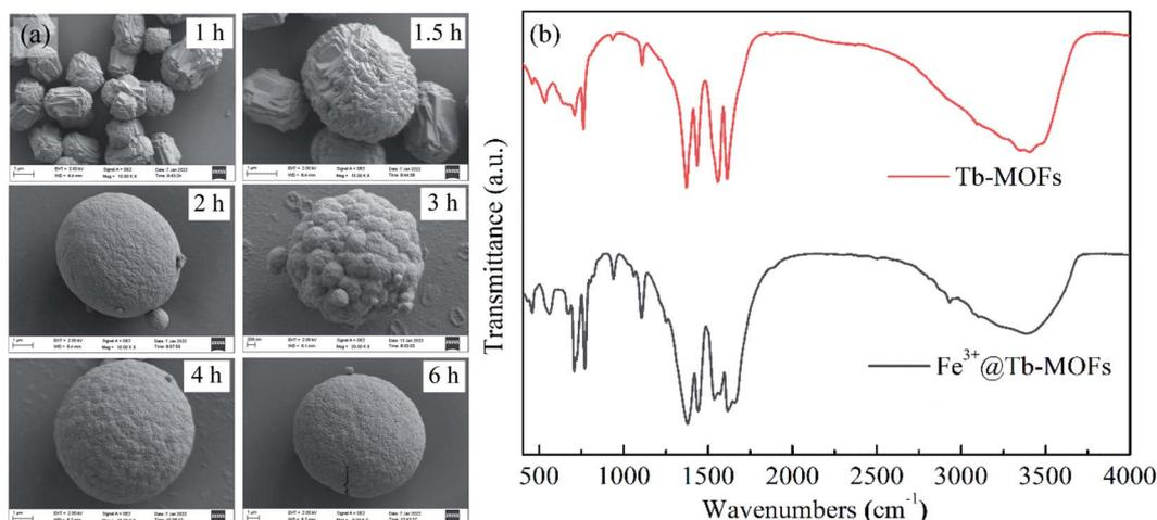
Fig. 3 (a) SEM images for 1 h, 1.5 h, 2 h, 3 h, 4 h, 6 h during Tb-MOFs preparation. The synthesis process of Tb-MOFs hollow spheres. (b) FTIR spectra of Tb-MOFs and Fe<sup>3+</sup>@Tb-MOFs.
