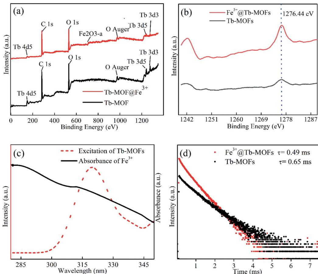
Fig. 5 (a) XPS spectra of Tb-MOFs and  $\text{Fe}^{3+}$ @Tb-MOFs. (b) Tb 3d XPS curves of Tb-MOFs and  $\text{Fe}^{3+}$ @Tb-MOFs. (c) UV-Vis spectrum of  $\text{Fe}^{3+}$  and excitation spectrum of Tb-MOFs, (d) Luminescence lifetime of Tb-MOFs and  $\text{Fe}^{3+}$ @Tb-MOFs.
