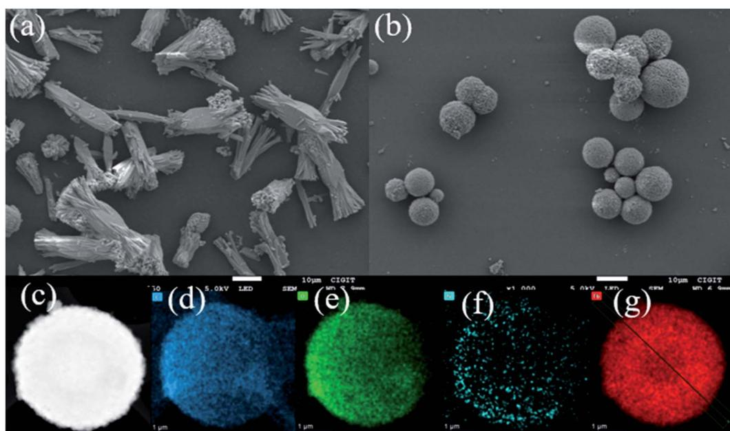
Fig. 2 (a) SEM image of Tb-MOFs without  $\text{H}_2\text{TDC}$ . (b) SEM image of Tb-MOFs with  $\text{H}_2\text{TDC}$ . (c) HAADF image of Tb-MOF with  $\text{H}_2\text{TDC}$ . (d)–(g) mapping images of C, O, N and Tb element, respectively.
