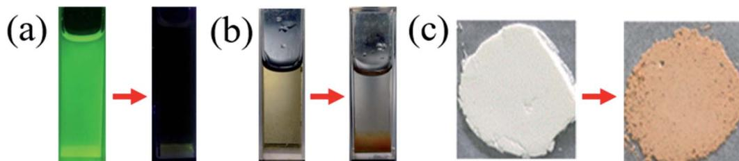
Fig. 6 (a) Photographs of Tb-MOFs suspension (left) and  $\text{Fe}^{3+}$  (right) under 365 nm illumination. (b) Photographs of  $\text{Fe}^{3+}$  before (left) and after (right) addition of Tb-MOFs. (c) Photographs of Tb-MOFs powder before (left) and after (right) adsorption of  $\text{Fe}^{3+}$ .
