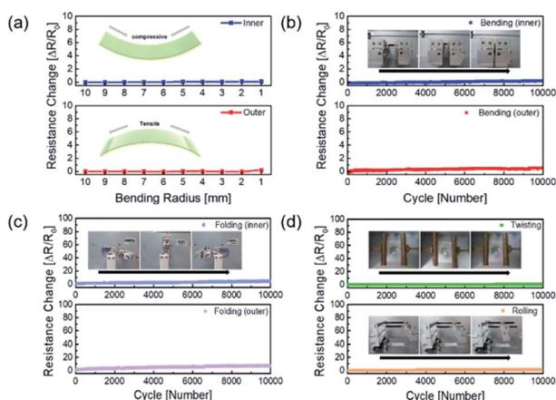
Fig. 5 (a) Resistance changes of AP electrode during bending test with decreasing bending radius, (b) inner and outer bending fatigue test for 10 000 times of cycles at a bending radius of 2 mm. (c) Inner and outer folding fatigue test for 10 000 times of cycles at a folding radius of 3 mm. (d) Twisting fatigue test with a twisting angle of 35° and rolling fatigue test at a rolling radius of 3 mm for 10 000 times of cycles, respectively.
