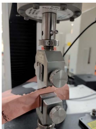
Fig. 2 Gross view image of the 180° peeling test.
