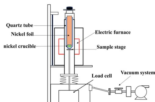
Fig. 1 Schematic diagram of self-designed thermogravimetric evaporation furnace.
