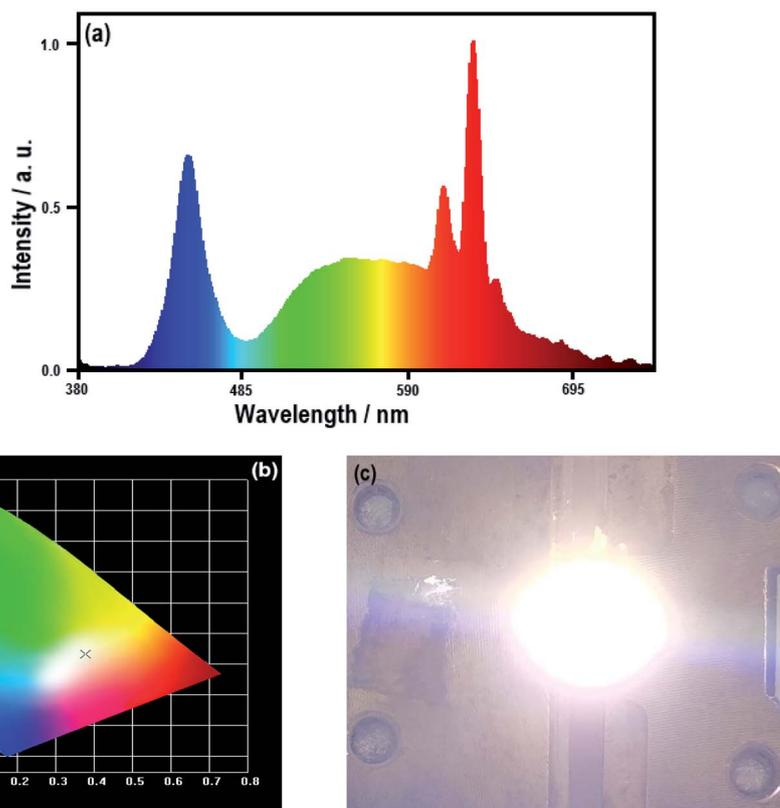
Fig. 6 Performances of prototype WLEDs using the mixing phosphors of  $\text{KTF} : \text{MEAH}^+, \text{Mn}^{4+}$  and  $\text{YAG} : \text{Ce}^{3+}$  based on InGaN chip under a 20 mA drive current: (a) electroluminescent spectra, (b) CIE chromaticity diagram, (c) luminescent photo.
