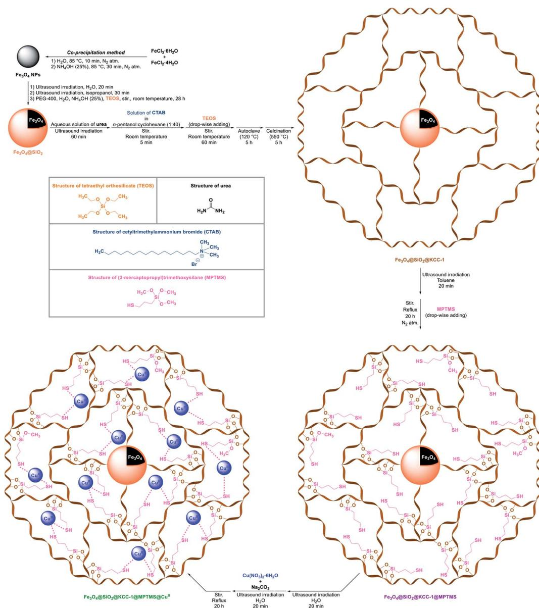
Scheme 1 Preparation of the cockscomb flower-like  $\text{Fe}_3\text{O}_4$ @ $\text{SiO}_2$ @KCC-1@MPTMS@ $\text{Cu}^{\text{II}}$  mesoporous nanocomposite.
